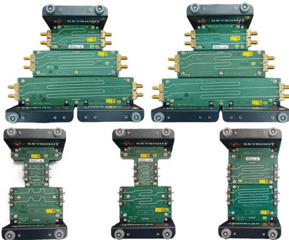
Figure 24. Keysight offers ISI channel boards M8067A-001, -002, -003, -004, and -005. The boards -001 and -002 offer 1.85 mm connectors and are suitable for emulating channel losses to characterize receivers that operate up to 64 GBd. For characterizing receivers that operate at symbol rates above 64 GBd and up to 120 GBd we recommend using the ISI channel boards M8067A-003, -004 or -005 with 1.00 mm connectors.
