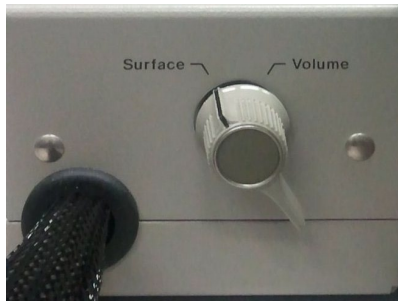
Figure 5. Selector switch of the N1424 Volume/Surface selector box
