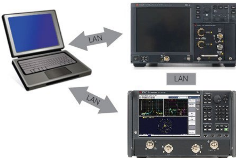
Figure 8. PC runs both DCA time-equivalent oscilloscope and PNA via LAN
