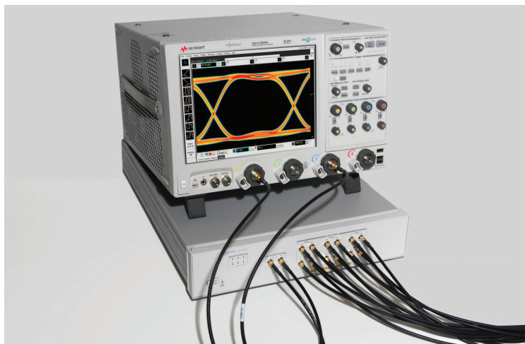
Figure 9. Automated testing for multi-lane digital bus interface through switching solution
