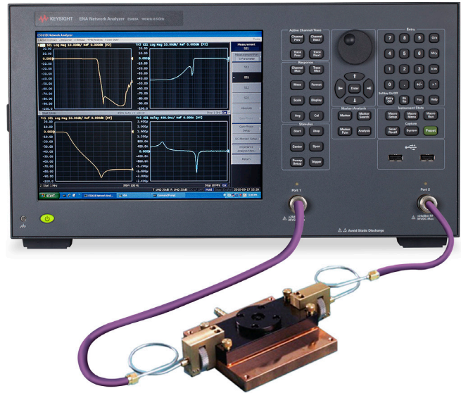
Dielectric properties measurements of PCB materials using the E5063A and N1501AExx test fixture
