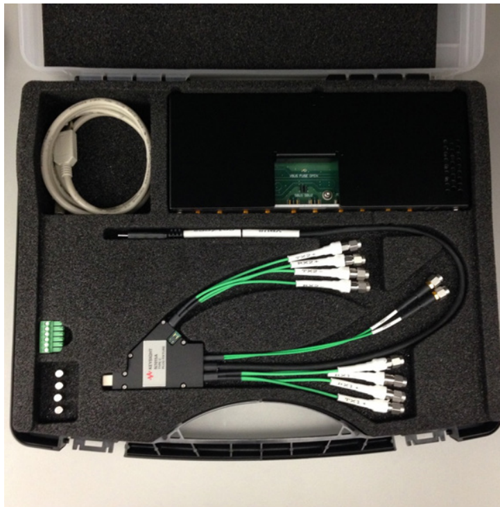
Figure 22. The Keysight N7015A USB Type-C Test Point Adapter Fixture.
