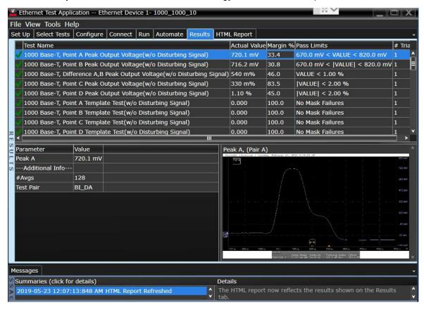
**Figure 5.** The D9010ETHC 10M/100M/1GBASE-T with Energy Efficient Ethernet compliance test application software results screen shows a summary of the tests performed, pass/fail status, and margin. Hyperlinks direct you to the more details of that test.
