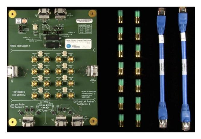
**Figure 9.** The EEE-TPA-ERK Wilder Technologies Energy Efficient Ethernet test fixture allows you to test to the 10BASE-Te, 100BASE-TXe and 1000BASE-Te Energy Efficient Ethernet standards. Sold separately through Wilder-Technologies.
