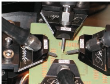
Figure 21. Step 2. Attach microprobes to the ends of the VNA cables Step 3. Perform all the measurements with microprobes
