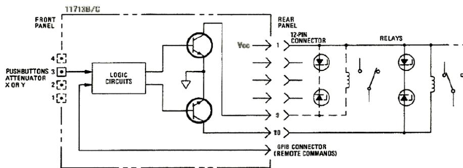
**Figure 2-7** Typical connection for relay driving circuit
