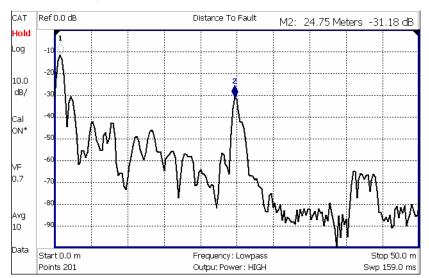
Figure 12-1 Marker 2 is Active, marker 1 is NOT active.
