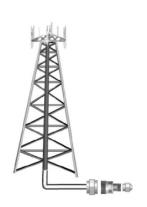
CAT Mode is typically used to test an entire transmission system, from the transmitter to the antenna. This process is sometimes referred to as Line Sweeping.
