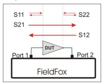
The FieldFox automatically switches the internal source and receivers to make both forward and reverse measurements. Therefore, the FieldFox can measure all four S-parameters with a single connection
