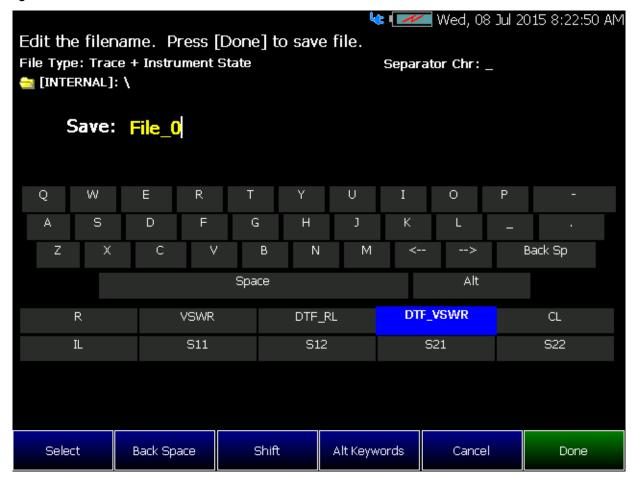
In the graphic above, the current filename is File\_0. The cursor is on the custom DTF\_VSWR keyword. The file will be saved to USB (flash drive). File Type is "Trace + State" (Instrument State).
