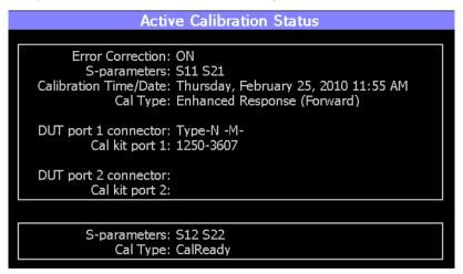
The top box shows the properties of the current calibration that you performed and the displayed S-parameters that it is correcting.
