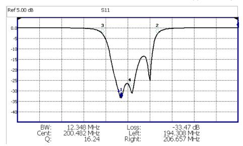
Press **Enter** and four markers are automatically created to find the first negative or positive bandpass over the displayed frequency range.
