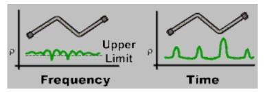
The frequency domain of an S11 measurement shows reflections caused by mismatches in the cable. It is impossible to determine where the mismatches physically occur in the cable.
