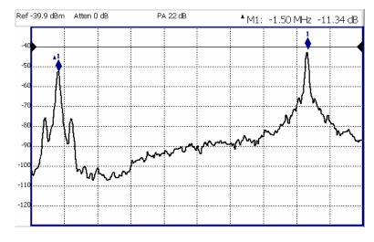
In the graphic above, the marker readout shows the difference between the two markers in frequency and amplitude.
