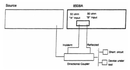
The above block diagram requires an external source and directional coupler to measure the electrical length of a DUT or cable to be trimmed. Separate paths are used to measure the Incident signal (A) and Reflected signal (B). To measure the ratio of the Reflected/Incident signals, you were required to select B/A for both the Magnitude and Phase display.
