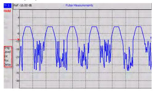
In the previous graphic, the settings are: Trig Level = -10 dBm, Trig Type (Int), Pos Slope (/), Delay
