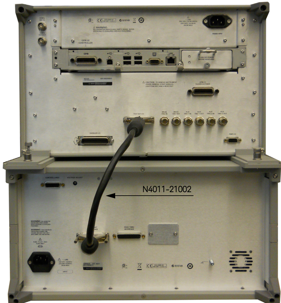
Figure 11 Test Set I/O Cable Connection
