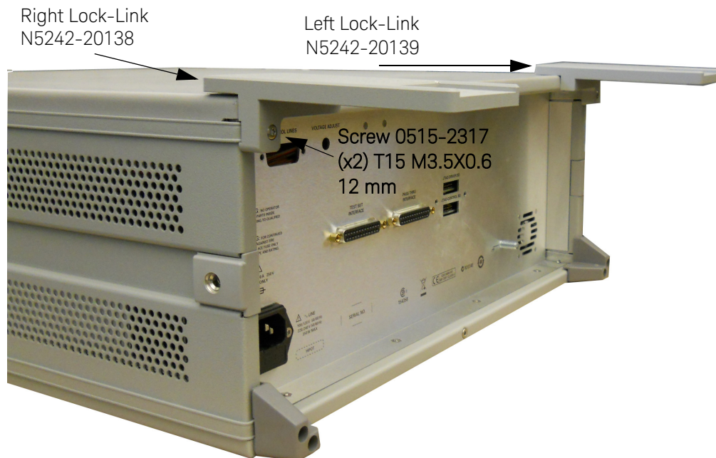
Figure 7 Install Lock-links to the Test Set
