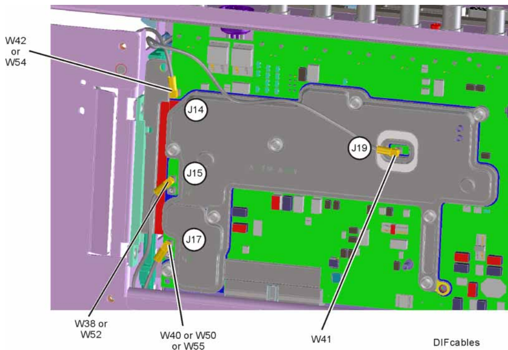
Figure 14-24 AIF/DIF Cables, bottom - Options MPB, B40, or DP2
