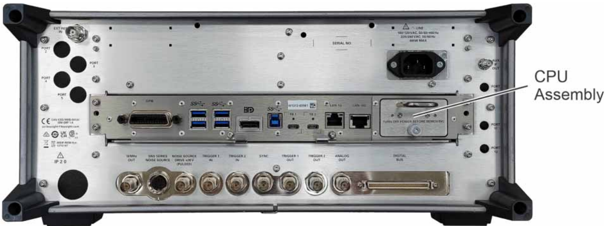
Figure 15-57 CPU Assembly - Rear Panel View
