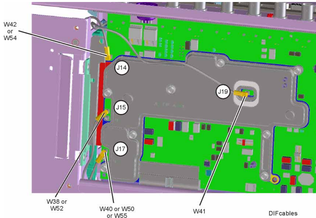
Figure 15-64 W38, W40, W41, W42 Removal - Option B40, MPB, or DP2
