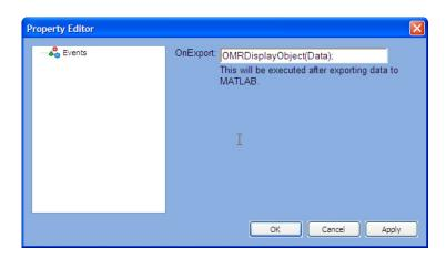
This plugin exports data directly into MATLAB. MATLAB needs to be installed on your computer. When you use this plugin, MATLAB will be started and the data will be transferred into the workspace. The data will be written into the variable "Data".
