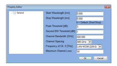
This plugin allows you to characterize filter transmission peaks. In a multi-channel measurement, one peak per channel will be detected and evaluated. So this is particularly adapted to measuring multiplexer passbands.
