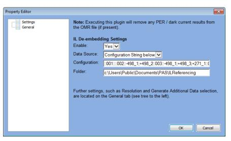
Measurement data generated by the IL/PDL engine can be re-evaluated if the measurement file contains raw data. In the IL/PDL engine, make sure "Keep Raw Data" is selected.
