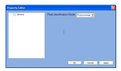
This plugin calculates the polarization dependent wavelength shift (often referred to as PD- $\lambda$ ). The plugin detects the difference of the peak center wavelengths of the TE and TM curve. Therefore, it can only run if the measurement contains a TE/TM graph. This plugin is licensed with the Filter/Multiplexer package.
