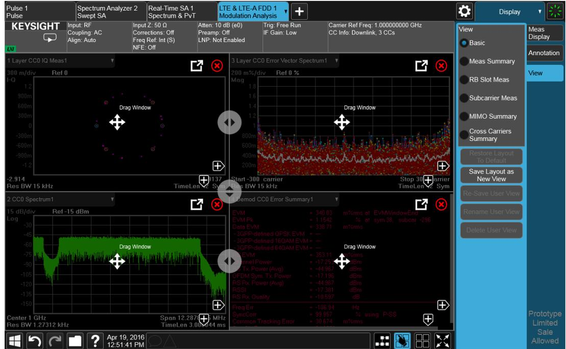
Each window has two arrows containing + signs. Pressing either of the “+” symbols adds a new window on that side. For example, let’s say you press the + symbol on the right of the lower left window:
