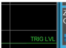
If the value of trigger level is off screen low this line displays along the bottom of the graticule. If the value of trigger level is off screen high this line displays above the graticule but no farther above than 1.5 % of the graticule height (the same as the trace itself). Note that the **TRIG LVL** label cannot display above the graticule so the label itself stops at the top of the graticule.
