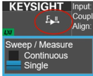
The **F** indicates that the instrument is using data from a file (if you wish to return to looking at data at the analyzer input, change the **Data Source** control in the **Input/Output, Data Source** menu from **File** back to **Input**.)
