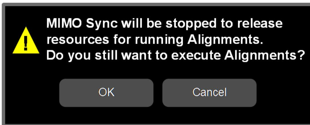
If the instrument is in MIMO sync, and you send a SCPI command to run Alignments, the align process is not executed, and a warning is generated. To execute Alignments, you must first stop MIMO via SCPI (or manually).
