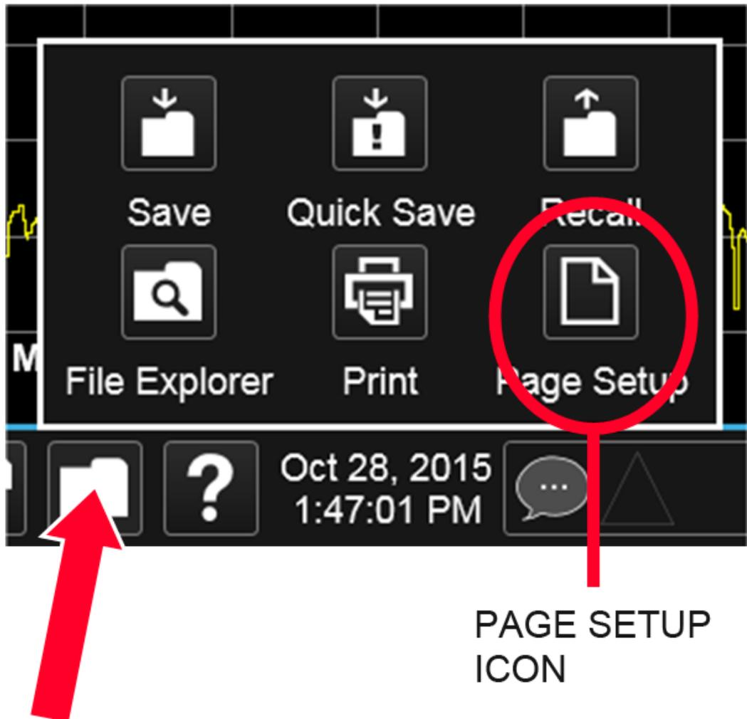
Opens a Windows Page Setup dialog that allows you to control aspects of the pages sent to the printer when the **PRINT** hardkey is pressed.
