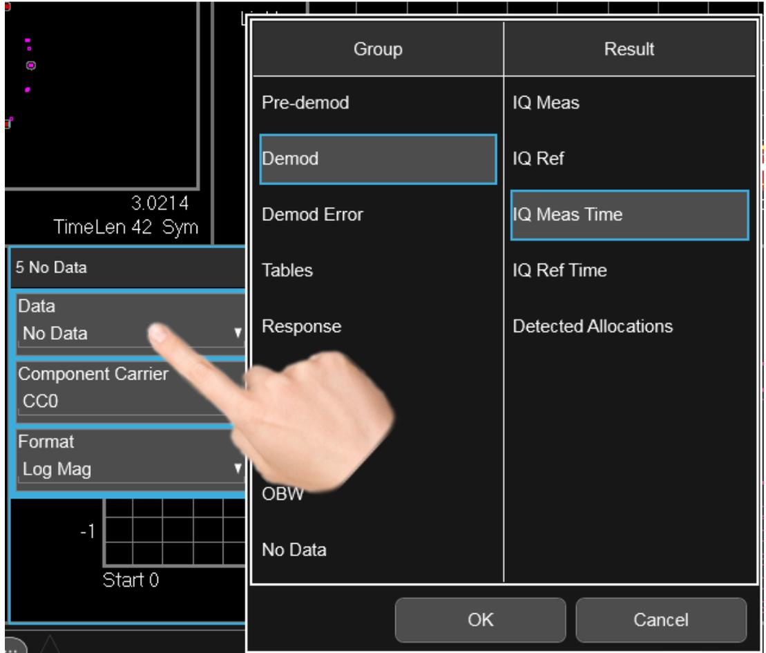
Note also that the Window Data dropdown sometimes includes controls for further configuring the window, for example, in LTE choosing the desired Component Carrier and Data format.
