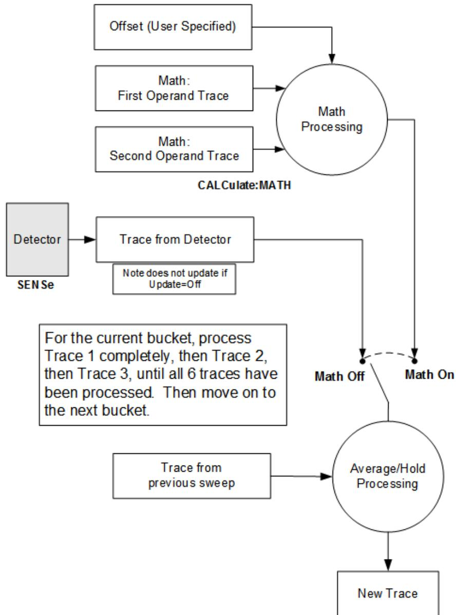
For the current bucket, process Trace 1 completely, then Trace 2, then Trace 3, until all 6 traces have been processed. Then move on to the next bucket.
