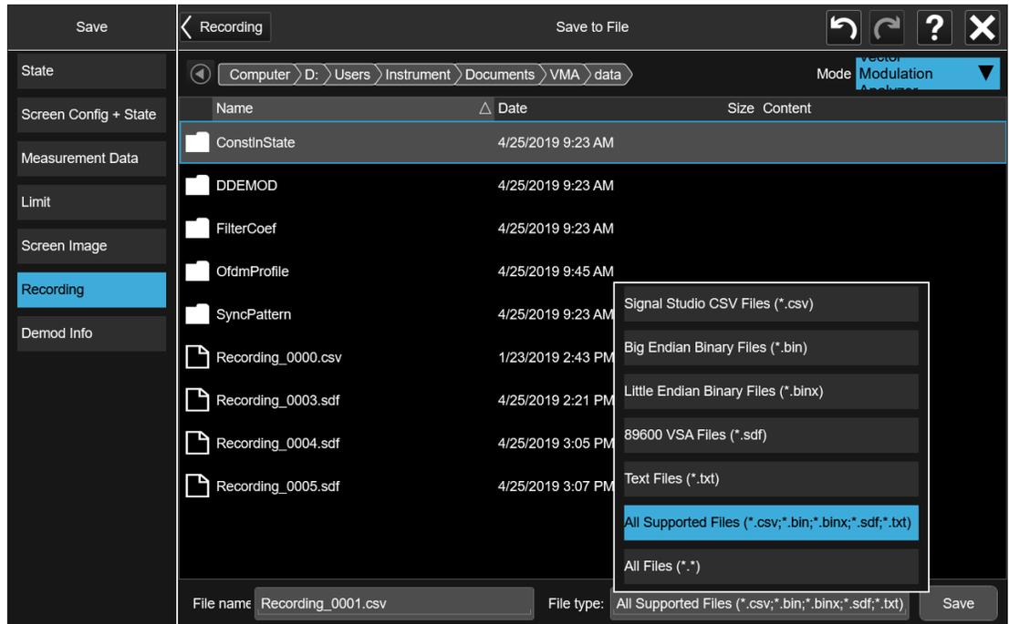
Then press **Save** to save the raw I/Q data of the current measurement.
