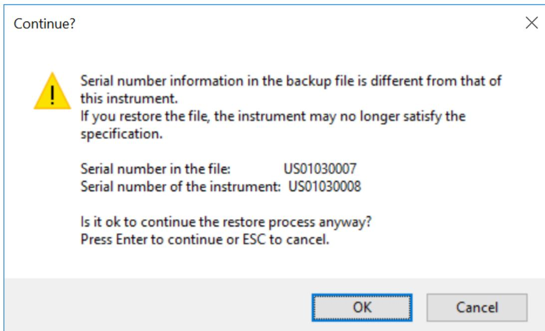
The default restore location for instruments *without* internal flash will be the first drive identified as an external drive (USB or LAN) if such is available; or, if not, the internal D: partition. The default restore file will be the most recent file that matches the default backup file name format: `<model number>_<serial number>_<date>.bkz`
