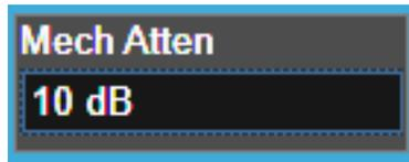
**Mech Atten** also appears with no switch, as above, in configurations that include an Electronic Attenuator but when the Electronic Attenuator is enabled.
