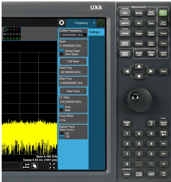
It is important to note that you can always pop up the Numeric Entry Panel by touching an active function control while it is active; for example, if you were to touch it in the figure above, the Numeric Entry Panel would pop up right next to the control:
