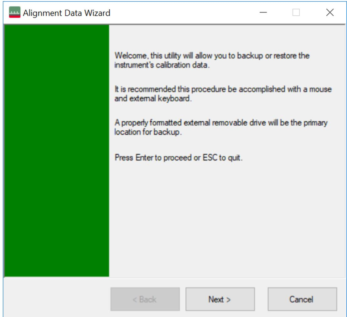
If your instrument has Processor Assembly type PC6S or PC7S (see ["Show System" on page 3087](#)) the instrument has an internal flash EEPROM that can store a backup of the alignment data. In this case, the interface to the Alignment Data Wizard is enhanced to accommodate this internal storage. This section details the use of this internal flash. For details on using external storage, see the previous section (["Alignment Data Wizard \(without Flash\)" on page 3203](#)).
