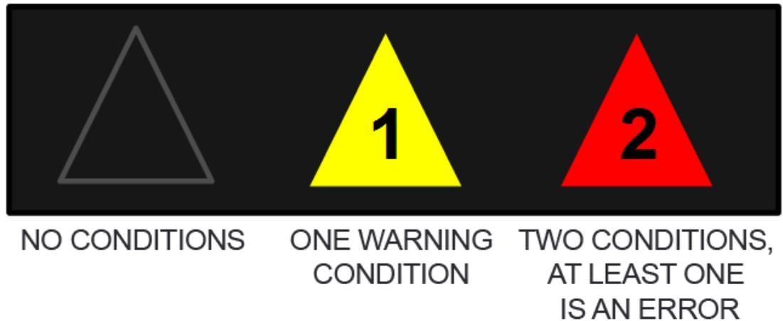
The triangle is unfilled if there are no open conditions, filled with yellow if all open conditions are warnings, and filled with red if at least one open condition is an error. The number displayed is the total number of open conditions.
