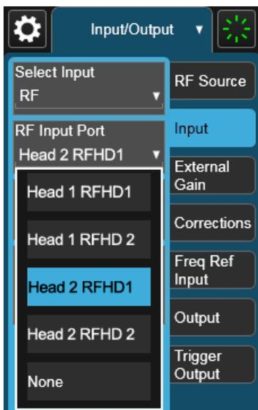
Note the inclusion of the **None** choice, which allows the input port to become unassigned, and thus allows any Output port to be assigned without concern about an Input port conflict. When the input port is unassigned, an error appears in the status area:
