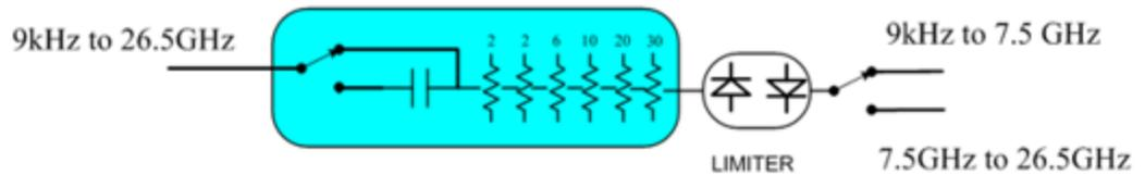
Note that Configuration 2 is not strictly speaking a dual-section attenuator, since there is no electronic section available. However, it behaves exactly like Configuration 1 without the Electronic Attenuator Option EA3, therefore for the sake of this document it is grouped into the “Dual-Attenuator” configuration.
