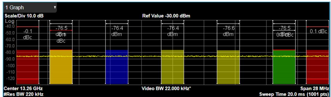
When the Bar Graph is **ON** and Limit Test is **ON**, the color of each bar graph reflects the limit test result. When the limit test fails, the bar color is red, and when limit test passes, the bar color is green.
