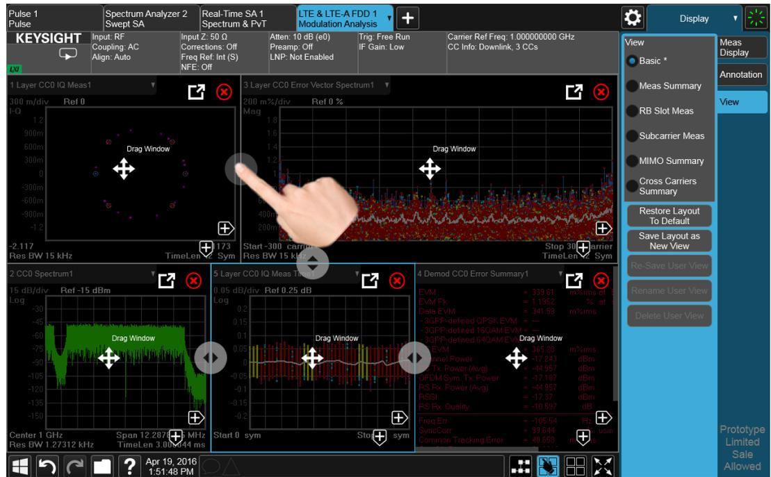
Another feature that comes with the View Editor is the ability to move windows around. You do this by dragging the four-arrow objects in the center of the window; the whole window goes along. Actually you can touch and drag anywhere in the window (except on one of the arrows or the delete circle) and it will drag, but the four-arrow objects give you an indication and a convenient finger target.
