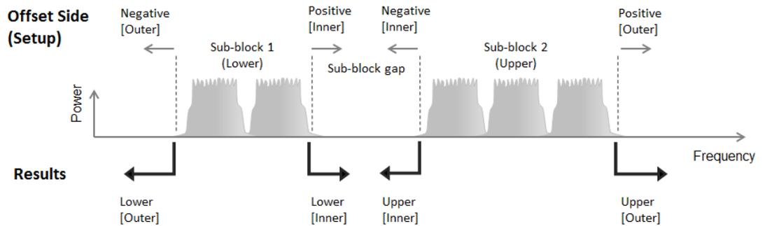
Remote Command `[ :SENSe]:SEMask:OFFSet[1]|2:INNer:LIST:SIDE BOTH | NEGative | POSitive, ...`
