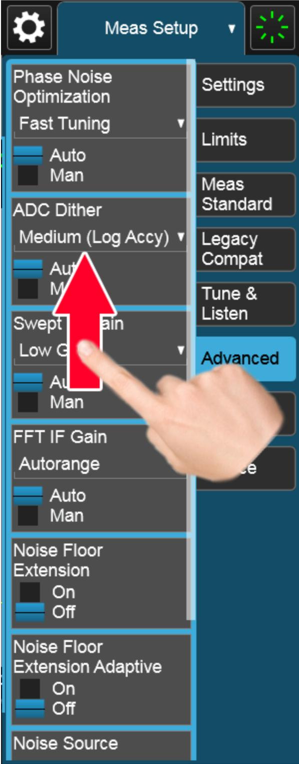
If you move to a different menu panel or sub-panel and then come back to a previous panel, the previous panel is always reset to be scrolled all the way back to the top.
