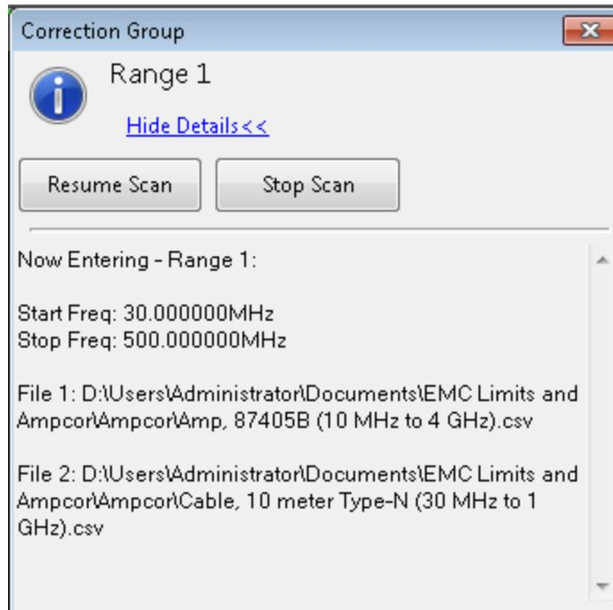
When running the Swept SA measurement in Spectrum Analyzer Mode, the message prompt is as below. You are given the option to resume the sweep or turn off the break. If in Continuous sweep, the sweep will resume after the break is turned off.
