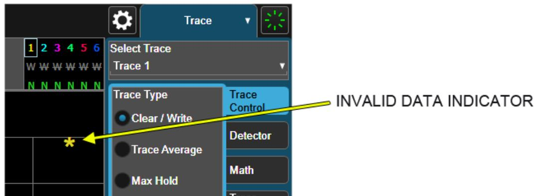
The Invalid Data Indicator is displayed whenever the data on the display does not match the settings of the instrument. The most common example of this is when instrument settings have changed in the time since the data in the traces on the display was taken. This means that the screen annotation cannot be guaranteed to match the trace data. For example, if you change **Center Frequency**, the Invalid Data Indicator will display until the trace has been retaken.
