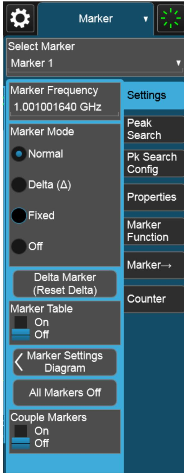
The menu panel normally appears on the right side of the display and consists of a rectangular panel with multiple “sub-panels” lying on top of each other, each sub-panel being accessed by a tab on the right.
