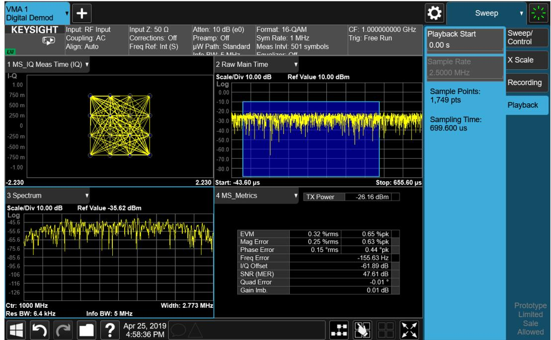
Note that the **Sample Rate** key is grayed out if the file type you loaded contains Sample Rate information. **BIN** and **BINX** files do not include sampling rate information inside the file, so after recalling one of these file types, you will need to set the Sample Rate. You should have noted the Sample Rate that was displayed on the **Sweep, Recording** menu panel after you saved the file.
