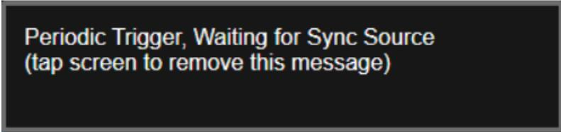
Once RF burst signal is provided and the hardware synchronized, the register will be cleared and a “Periodic Trigger Synchronized” message will be generated.
