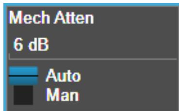
Note that in configurations that include an Electronic Attenuator, this switch is only shown when the Electronic Attenuator is disabled.
