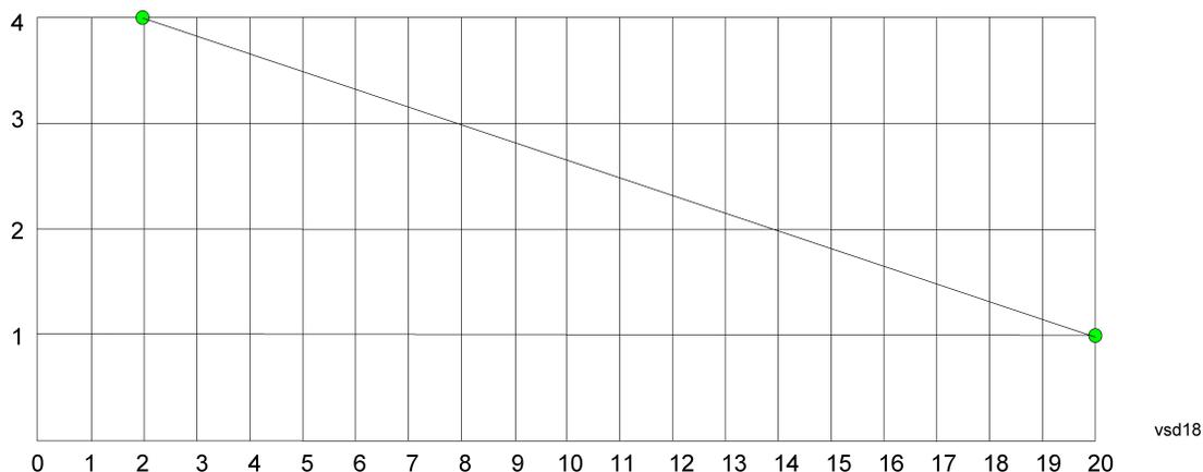
The correction to be used for each bucket is taken from the interpolated correction curve at the center of the bucket.
