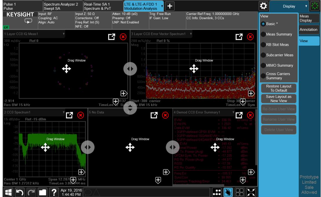
A fifth window has been added, and is automatically assigned the number 5. (The window number, which is displayed in the Window Title region, is used when sending SCPI commands to that window).
