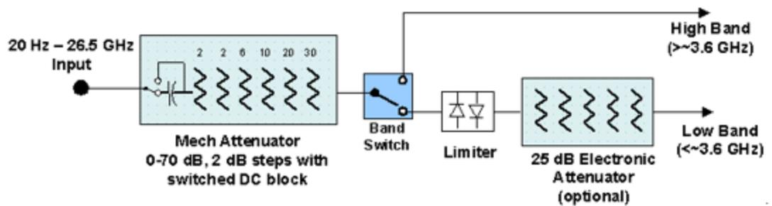
Configuration 2: Mechanical attenuator, no optional electronic attenuator
