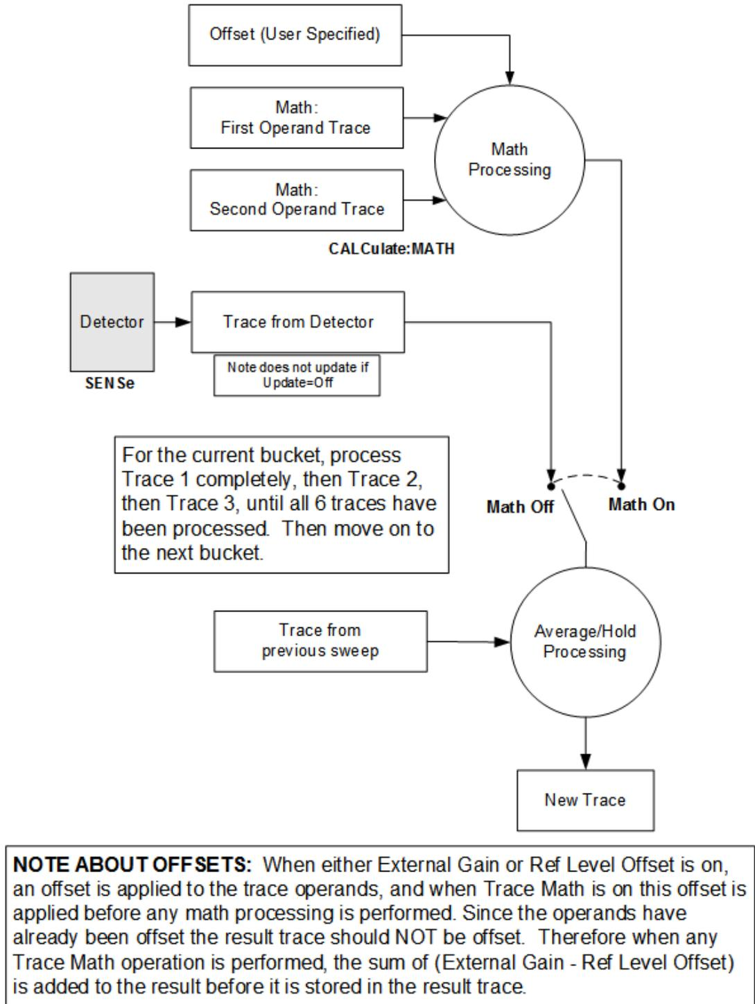
For each active trace, the current trace point is processed for **Trace 1**, then **Trace 2**, then **Trace 3**, etc. Trace data is taken from either the detector for that trace, or
