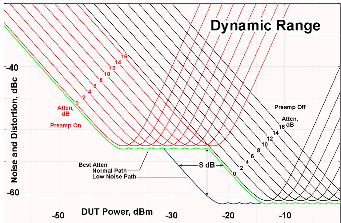
There are other times where selecting the low noise path improves performance, too. Compression-limited measurements such as finding the nulls in a pulsed-RF spectrum can profit from the low noise path in a way similar to the TOI-limited
