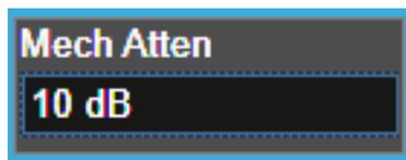
**Mech Atten** also appears with no switch, as above, in configurations that include an Electronic Attenuator but when the Electronic Attenuator is enabled.
