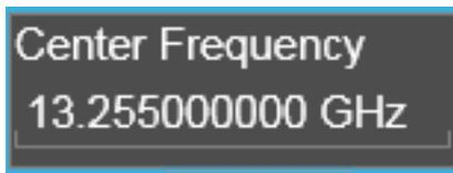
An active function is “active” if the numeric value is surrounded by a black background with a blue border, as below. In this state, it is ready to receive numeric input from the number pad on the front panel, the knob, or the step keys.
