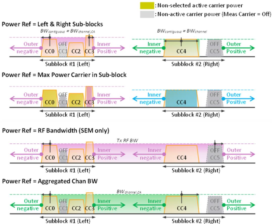
Remote Command `[[:SENSe]:SEMAsk:CARRier:PREFerence:TYPE LRCarriers | MPCarrier | CINDEX | MANual | MPCSubblock | RFBandwidth | ACBandwidth | LRSubblocks`
