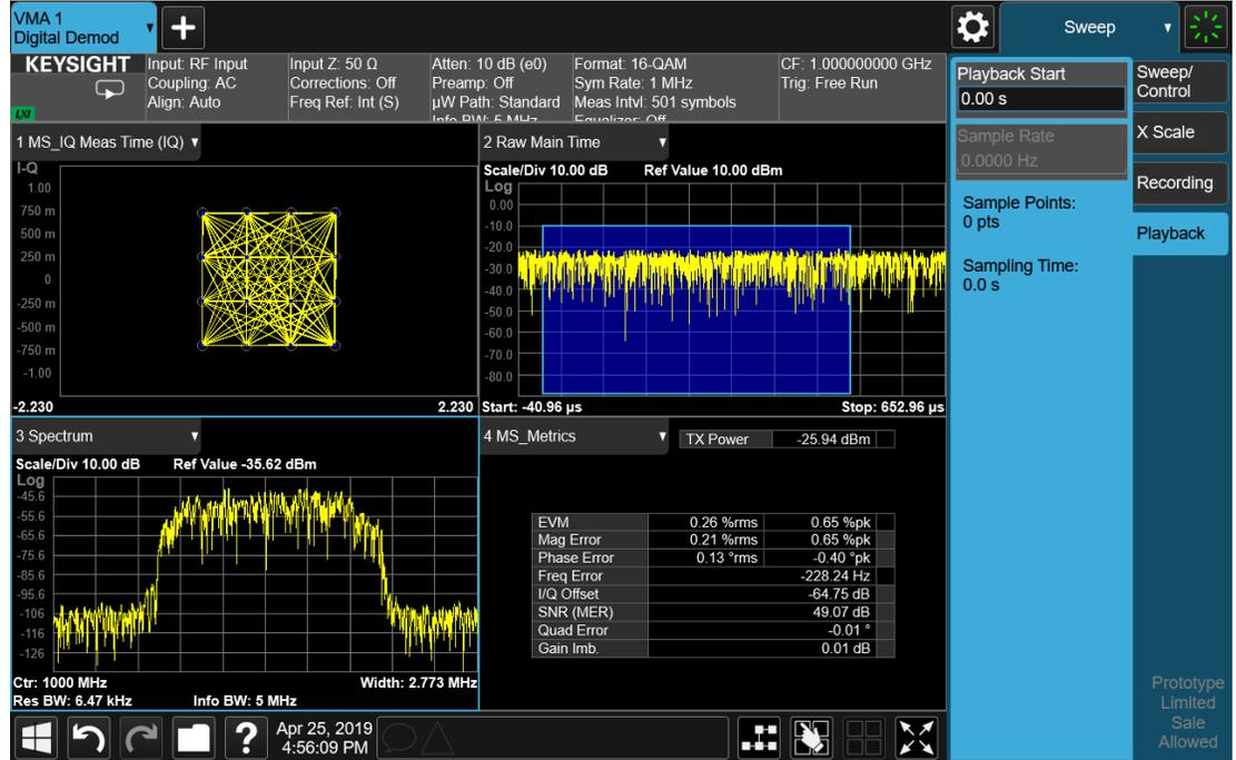
To recall a Recording, press the **Recall** hardkey (or the **Recall** icon in the **File** panel) and press the **Recording** tab on the left side of the **Recall** panel. Then press **Recall From** and choose the file you would like to recall. This will read the raw I/Q data from the specified file and feed it to the current measurement.
