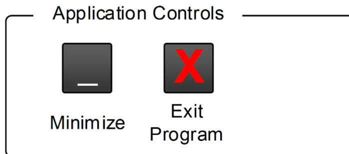
Pressing **Exit Program** displays a prompt asking if you are sure you want to close the program. If you select **OK**, the entire analyzer application will shut down, and you will lose any unsaved trace or measurement data.
