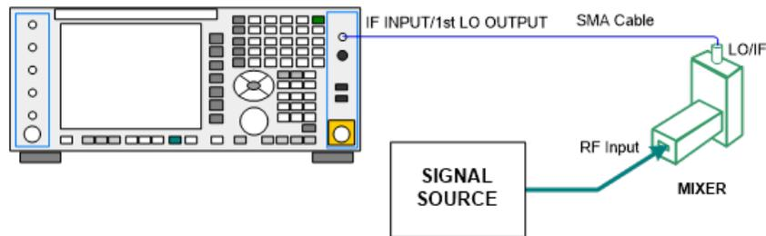
Legacy HP/Agilent and some third-party mixers have separate LO In and IF out connections. This requires you to use an external diplexer to connect these mixers. A diplexer can easily be purchased for this purpose (for example, Diplexer Model # DPL.26 or # DPL.313B from OML Inc., Morgan Hill, California, USA).
