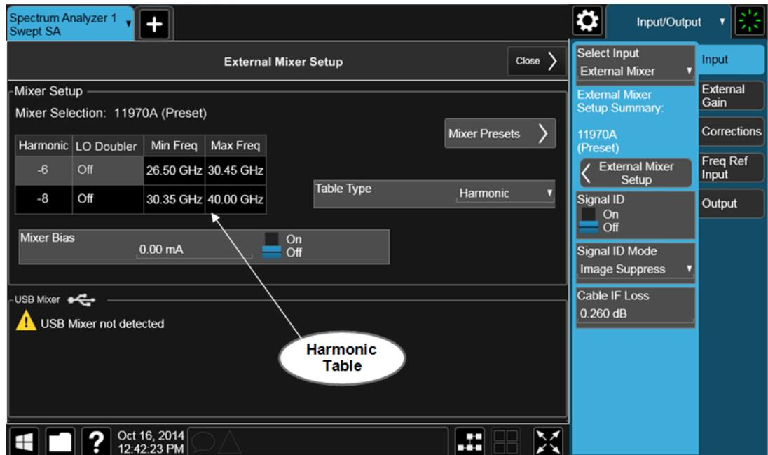
The current Mixer selection (the current or most recently connected USB Mixer, or the most recent Mixer Preset, or **Custom** if you have modified the setup) reads out at the top of this screen as **Mixer Selection**
