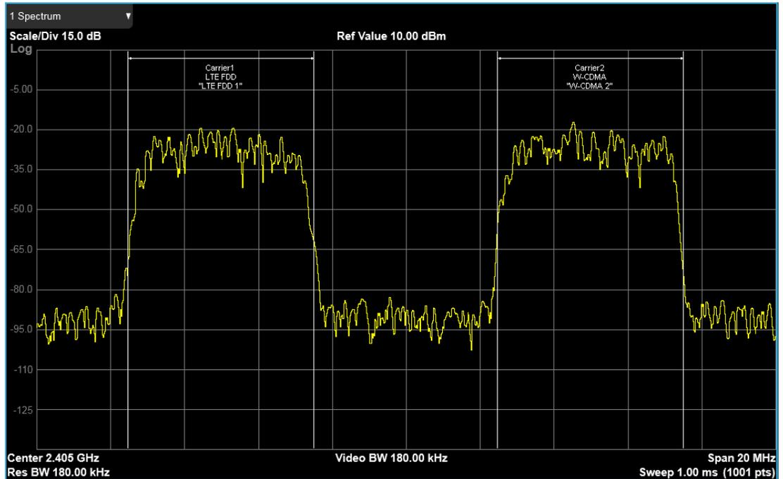
When Carrier and Sub-block attributes are both on, the sub-block scope and name are also shown on the spectrum trace:
