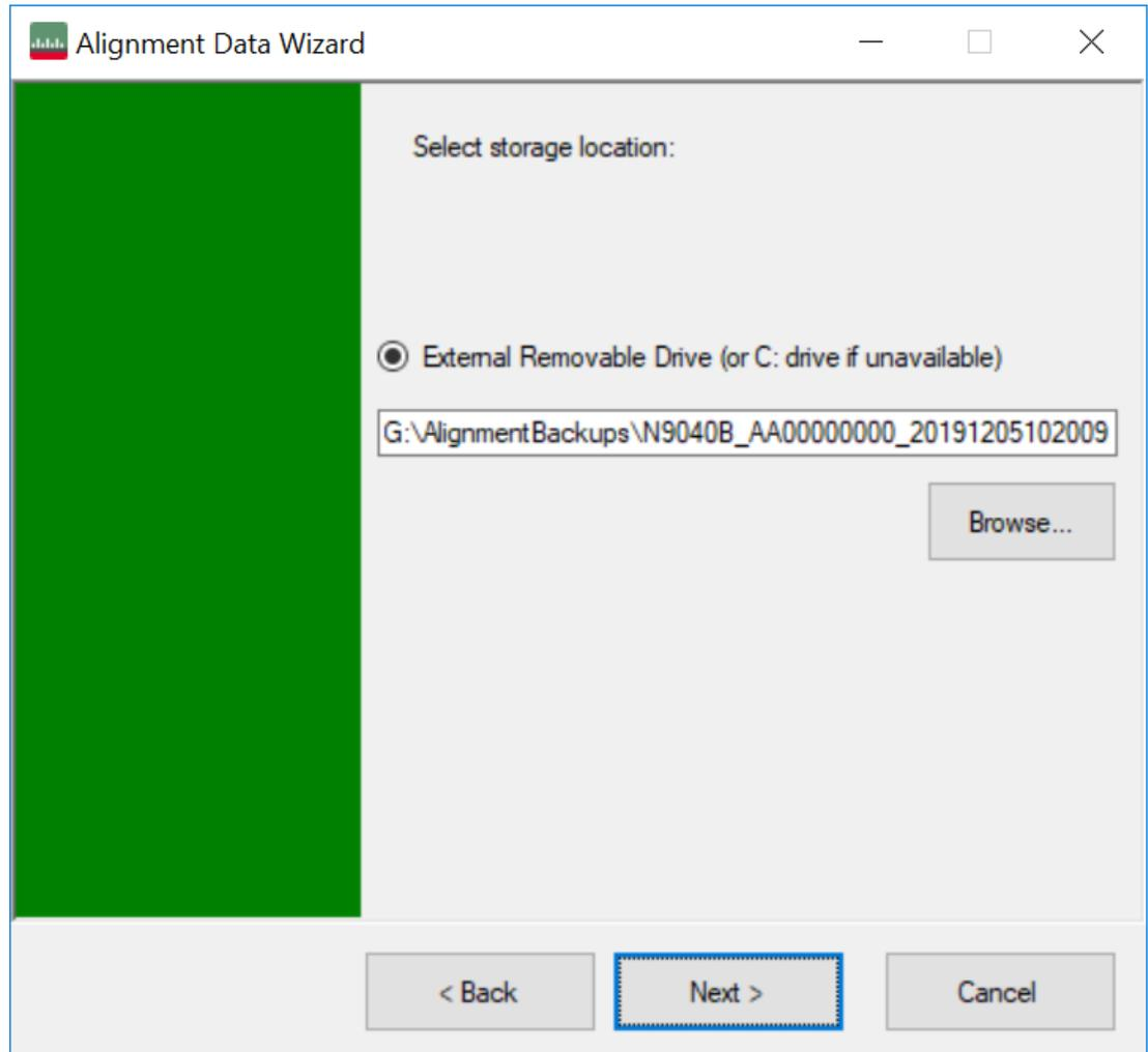
If a USB drive is present, it will be selected by default. The path defaults to the **AlignmentBackups** folder, and a filename is automatically created, in the form: `<model>_<serial number>_<date><time>.bkz`
