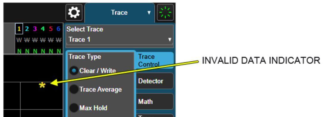
The Invalid Data Indicator is displayed whenever the data on the display does not match the settings of the instrument. The most common example of this is when instrument settings have changed in the time since the data in the traces on the
