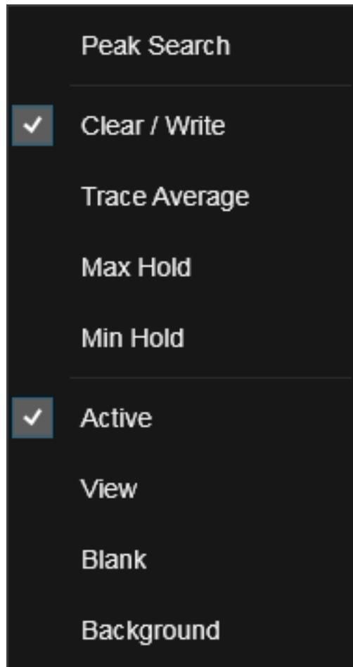
If you now tap or click on one of the items in this menu, the instrument will perform the corresponding function. **Peak Search** finds the highest peak on the selected Trace. **Clear/Write**, **Trace Average**, **Max Hold** and **Min Hold** set the "Trace Type" on [page 2927](#). **Active**, **View**, **Blank**, and **Background** set the "View/Blank" on [page 2932](#) type.
