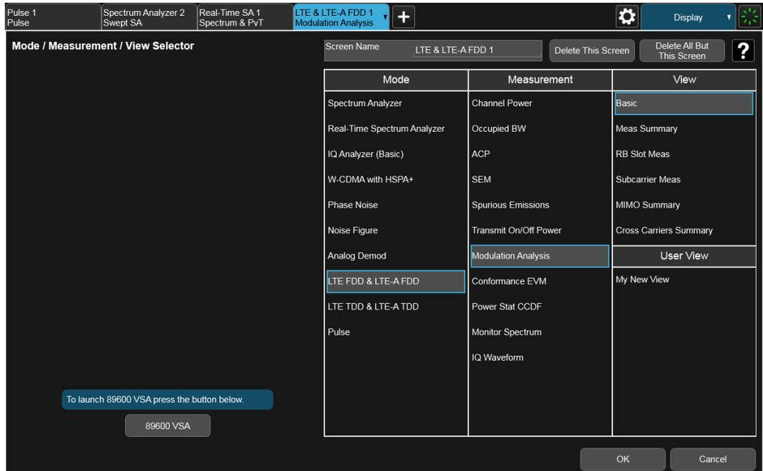
When naming a new View, you must choose a name that is not already in use for any User View in any measurement; this is because User Views get written to permanent memory and are available to all instances of the Measurement in any screen. They survive a Mode Preset and also survive shutdown and restart of the application.
