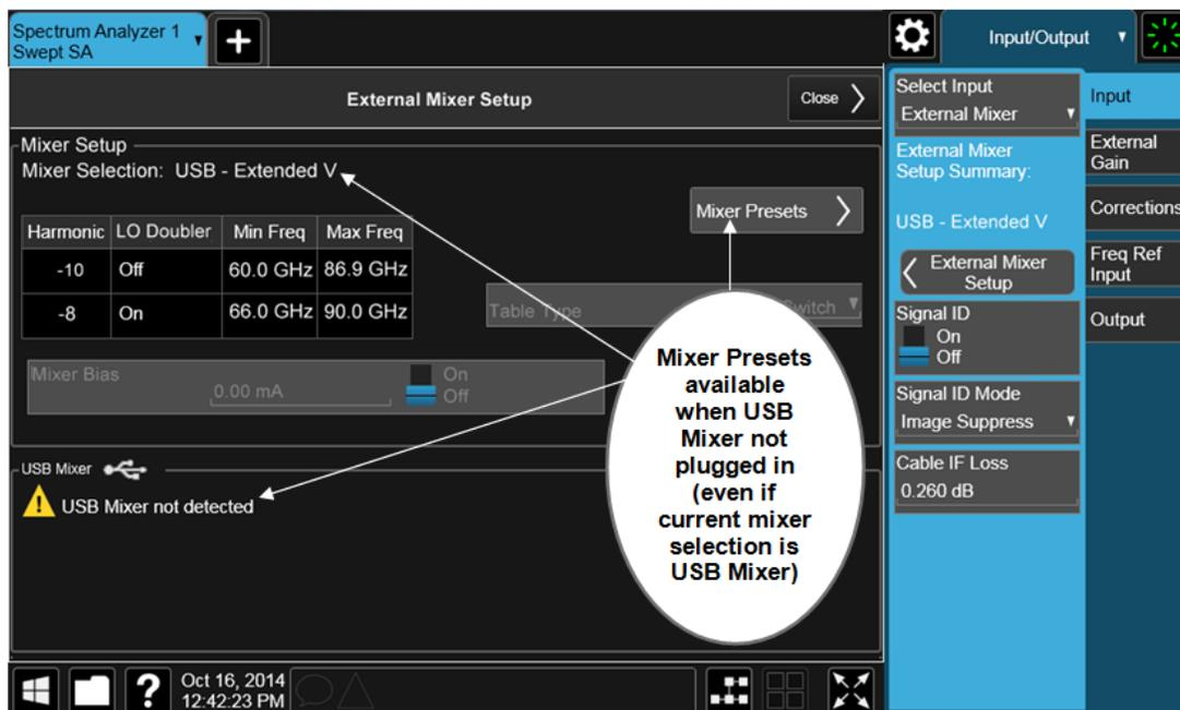
Only one USB Mixer is supported at a time. To switch to a different USB Mixer, disconnect the one that is no longer being used prior to connecting a new one.
