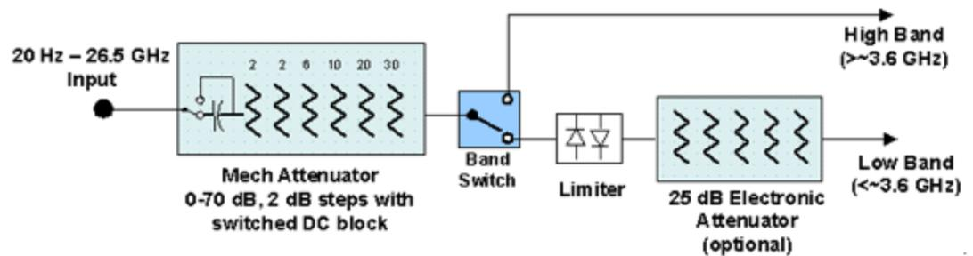
Configuration 2: Mechanical attenuator, no optional electronic attenuator
