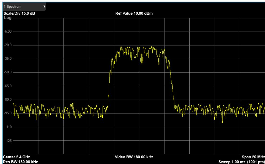
In **LTEAFDD/LTEATDD, MSR and 5G NR Modes**, multi-carriers are supported. The Carrier Attribute on/off and Sub-block Attribute on/off settings (under Display, Meas Display) are defined to allow the carrier and sub-block legends to display.
