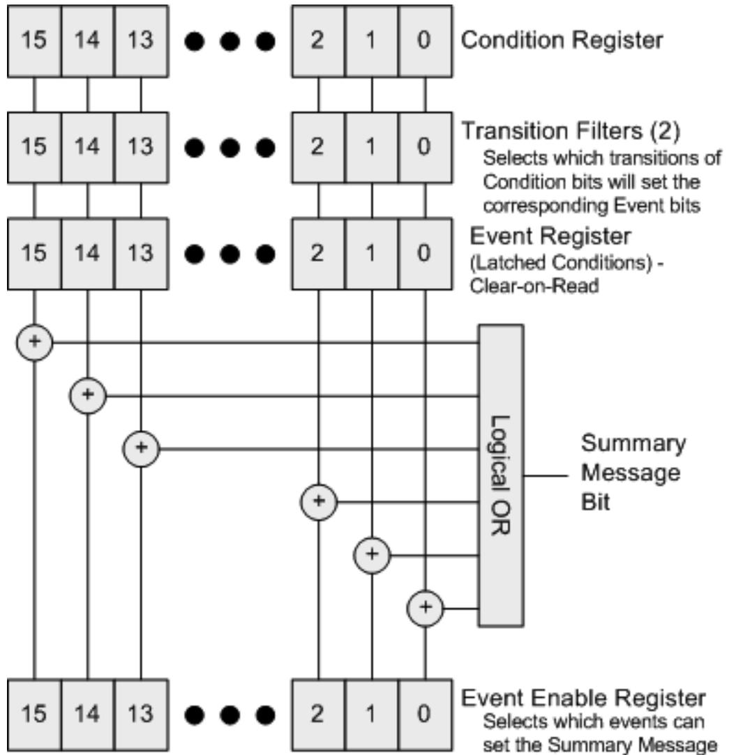
The settings of the Transition Filter registers determine whether or not a bit set in a Condition register ripples through to the Event register, as follows:
