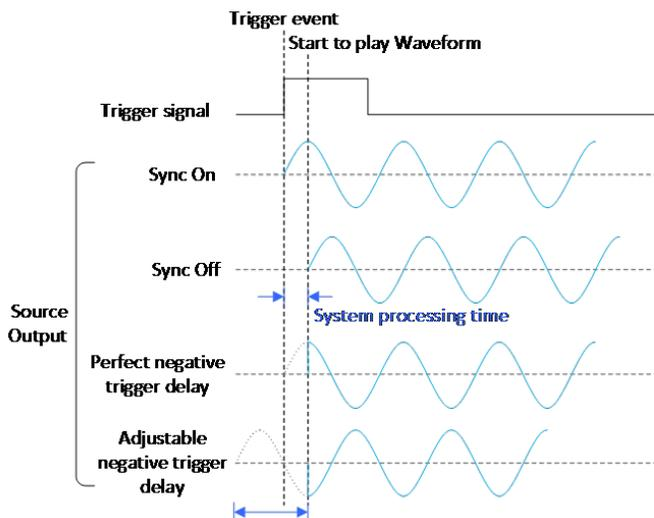
Note: the first PerArb trigger signal will be missed when the trigger delay is negative.
