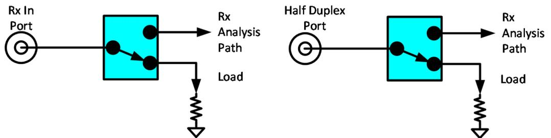
When using Source only, set RF Input to **NONE** to provide better isolation. When the input port is set to **NONE**, an error appears in the status area:
