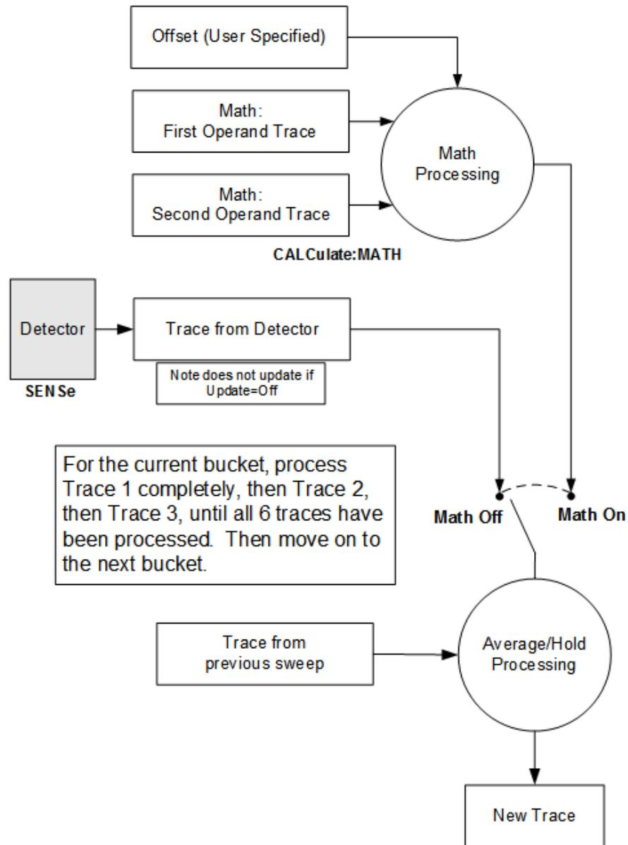
**NOTE ABOUT OFFSETS:** When either External Gain or Ref Level Offset is on, an offset is applied to the trace operands, and when Trace Math is on this offset is applied before any math processing is performed. Since the operands have already been offset the result trace should NOT be offset. Therefore when any Trace Math operation is performed, the sum of (External Gain - Ref Level Offset) is added to the result before it is stored in the result trace.
