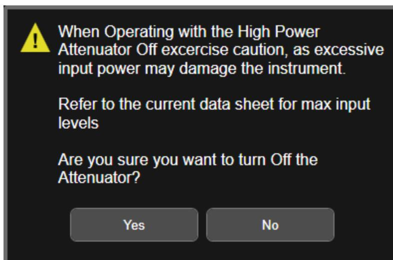
Whenever the attenuator is bypassed (**OFF**), a warning appears in the status bar: "Input caution; T/R unprotected"
