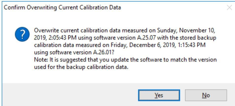
When backing up alignment data to the flash, if there is already an existing backup on the flash, a final confirmation message is displayed detailing what is being backed up and what will be overwritten on the flash (again, the dates and versions are examples):
