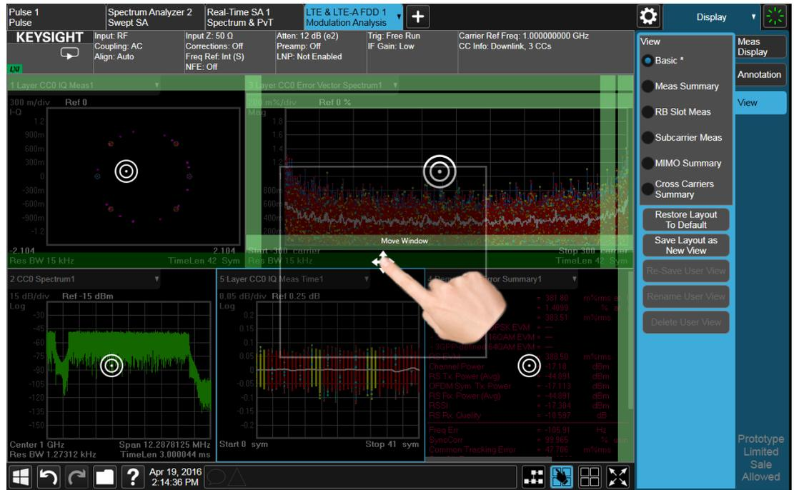
When you hover over one of the stripes it gets dimmer, to show the position the window being dragged will take on. If you release a window over an inner stripe, the window you are dragging and the window over which you were hovering resize to share the space the target window originally occupied. If you release a window over an outer stripe, as shown below, the window you are dragging takes on a new position outside the array of other windows:
