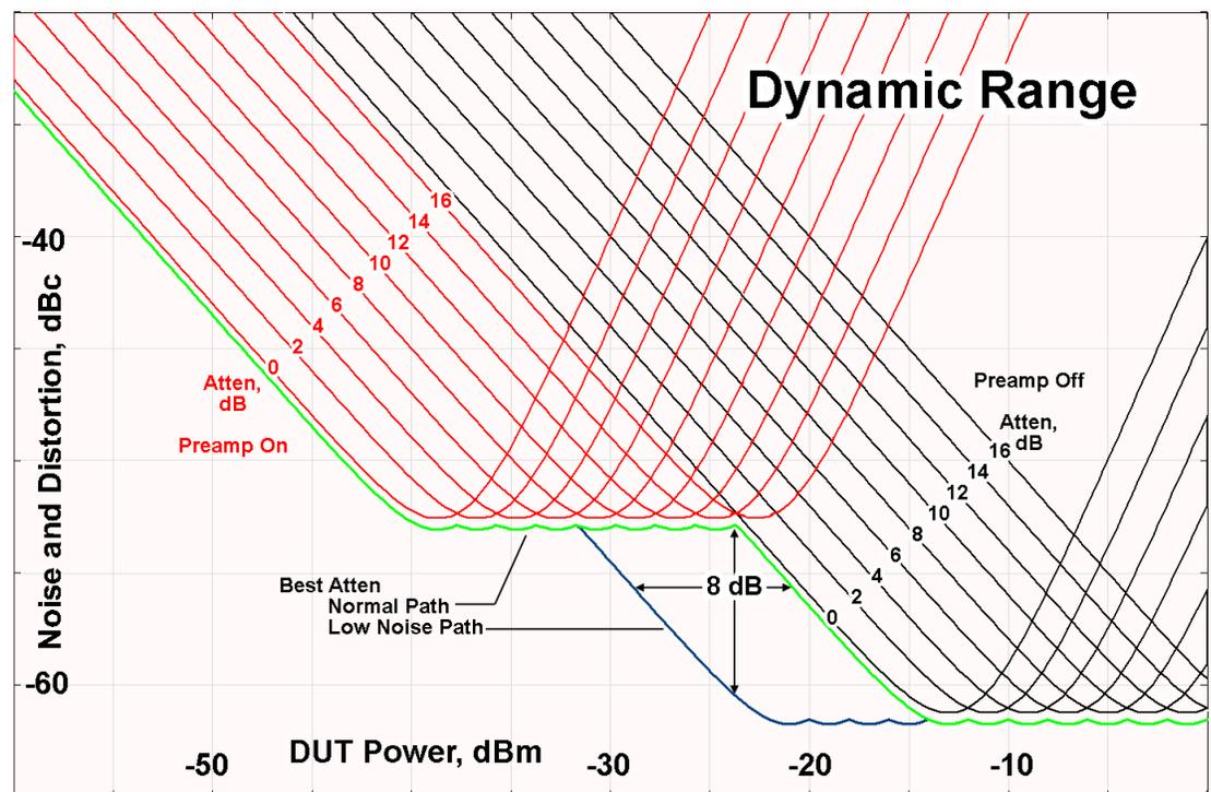
There are other times where selecting the low noise path improves performance, too. Compression-limited measurements such as finding the nulls in a pulsed-RF spectrum can profit from the low noise path in a way similar to the TOI-limited
