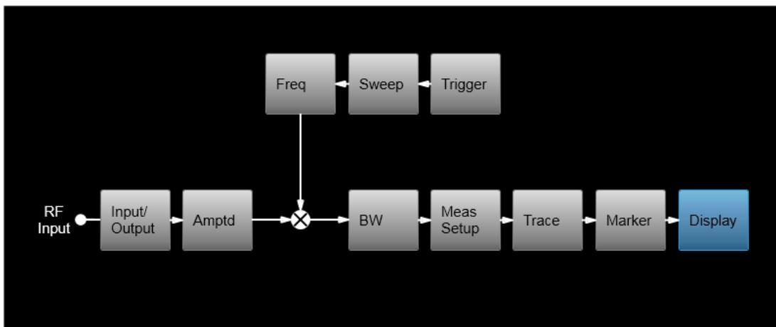
And here is the Block Diagram when External Mixing is selected:
