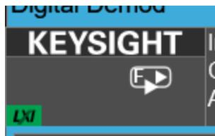
This indicates that the instrument is in **Continuous Playback** mode and is using data from a File.
