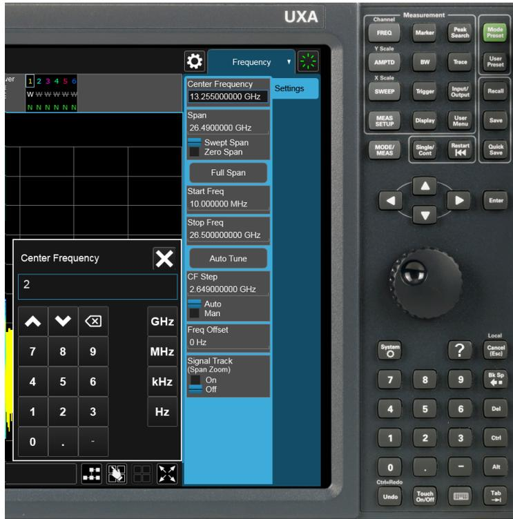
Type in as many digits as required, then touch one of the unit terminator buttons in the Numeric Entry Panel to complete the entry. In this case, 2 GHz was the desired entry, so you just touch the “GHz” terminator:
