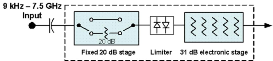
You can tell which attenuator configuration you have by pressing the Attenuation tab, which (in most Modes) opens the Attenuation menu. If the first control in the Attenuation menu says **Mech Atten** you have the Dual-Attenuator configuration. If the first control says **Atten** you have the Single-Attenuator configuration.
