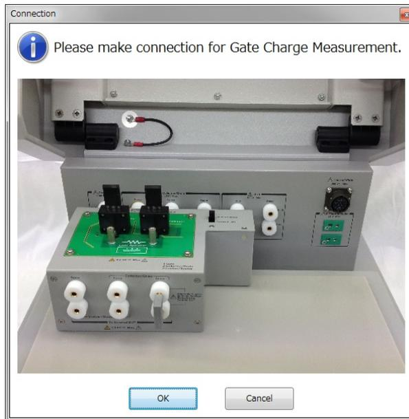
1. Open the test fixture cover and remove the accessory from the test fixture.
