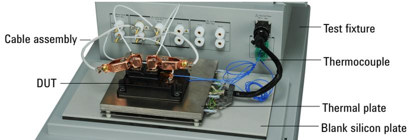
In the above picture, the blank silicon plate is set on the DUT stage of the test fixture, and the Thermal Plate is placed on the plate and connected to the Thermal Plate connector. Also, the thermocouples are connected to the K Thermocouple terminals and put on the places to monitor temperature. For the Thermal Plate, contact inTEST Corporation.
