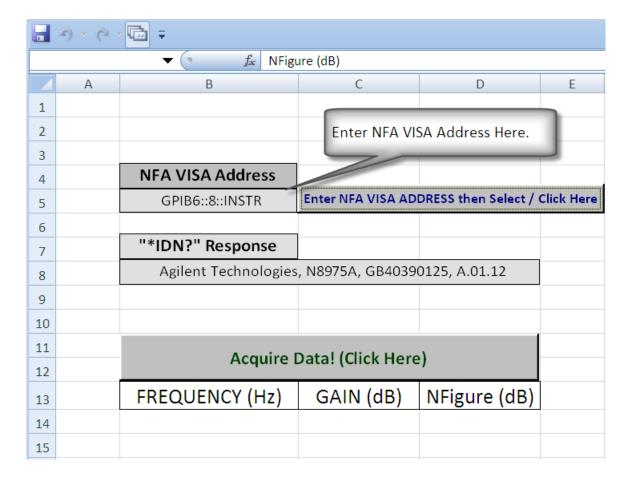
The VISA address is set and configured via the installation of the specific vendors I/O Libraries. The following view represents an Agilent I/O Libraries installation and the resultant Agilent Connection Expert (ACE) configuration with indications for this specific configuration and NFA connection.
