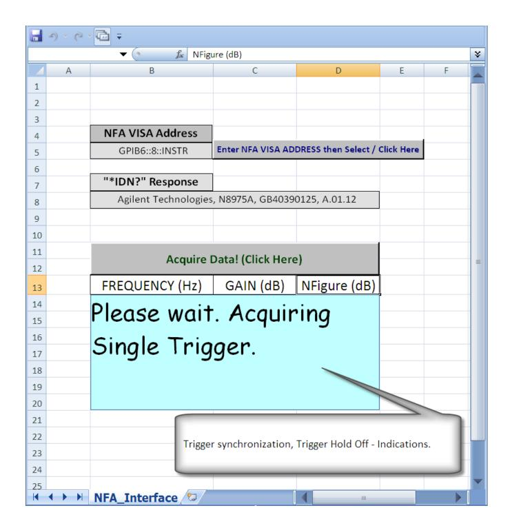
Upon completion of the single sweep the FREQUENCY (Hz), GAIN (dB) and NFigure (dB) columns are updated within the Excel spreadsheet and the trigger mode is returned to internal, continuous and free run on the NFA.
