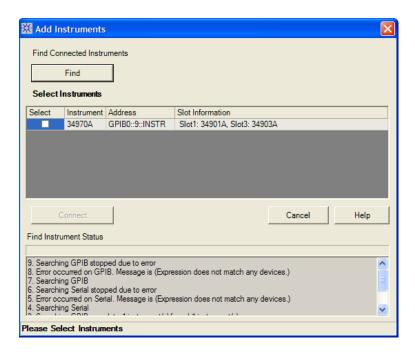
The **Find Instrument Status** area shows the status of the find operation. If you do not see any instruments listed, check that the interface is connected and the instrument is powered-on. For more information on troubleshooting configuration problems, refer to the Agilent Connection Expert application on the *Automation-Ready CD ROM* included with the instrument.
