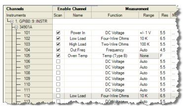
9 The More column under Measurement allows you to select advanced settings for the measurement function. For example, for the DC Voltage function, you can set Number of Power Line Cycles, Channel Delay and DC Input Resistance. For this tutorial, click ••• in the More column for channel 101, and set the Number of Power Line Cycles-NPLC to 10 and click OK. This sets the integration time for the DMM.
