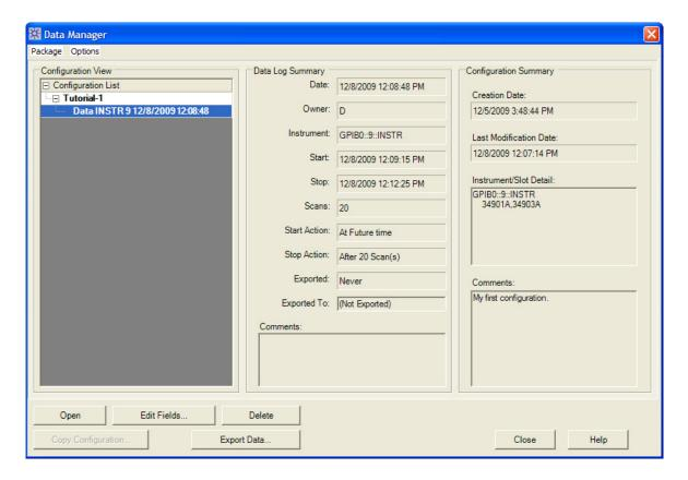
2 The Tutorial-1 configuration and the recently scanned data log should appear in the Configuration View column. With the data log selected as shown above, click the Export Data button. The Export Data dialog box appears and allows you to specify how to export the data and which data to export. For this tutorial, we will use the default export settings
