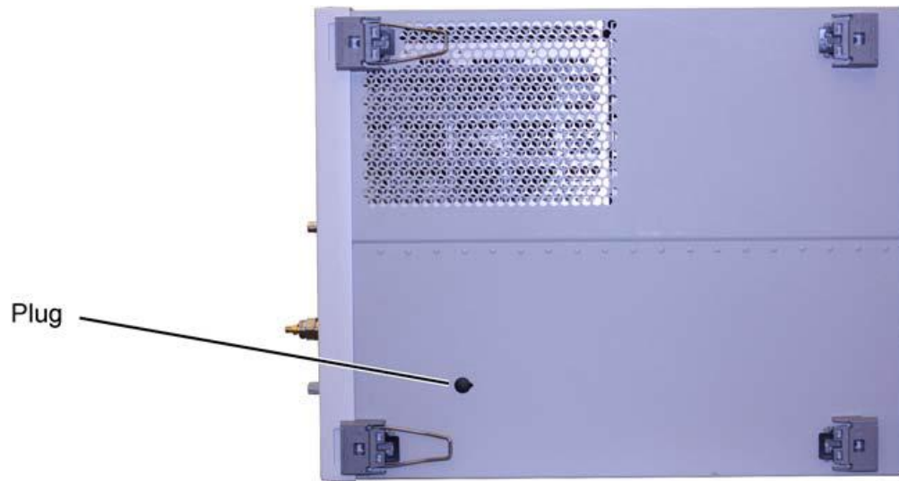
Figure 3. Removing the Timebase Adjustment Access Plug
