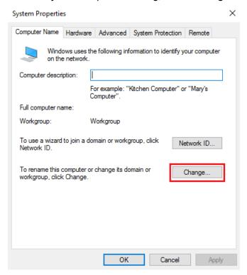
7. In the Computer Name/Domain Changes dialog, enter your desired Computer Name. (The default factory Computer name is K-M9384B-12345, where 12345 is the last 5 digits of the instrument's serial number.) Note that the Computer Name cannot conflict with the name of another device on your network.
