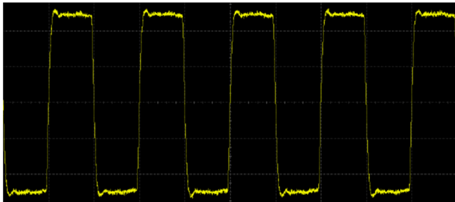
Figure 9-2 Typical Negative Droop Test Waveform (using a pair of SMA cables)
