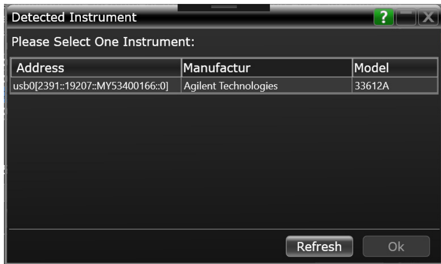
Figure 11-25 Adding the instrument to External instrument window.
