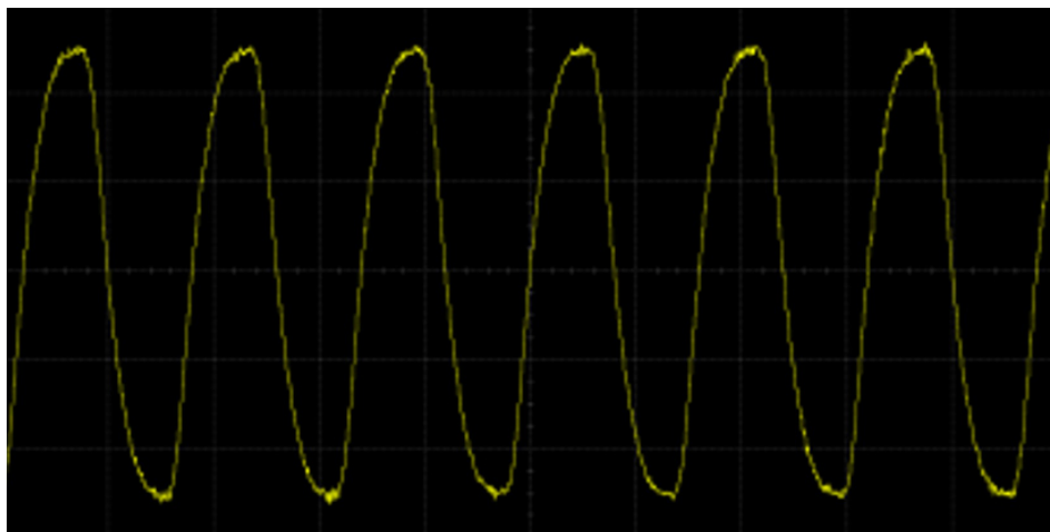
Figure 9-3 Typical Test Mode 2 Waveform (using a pair of SMA cables)
