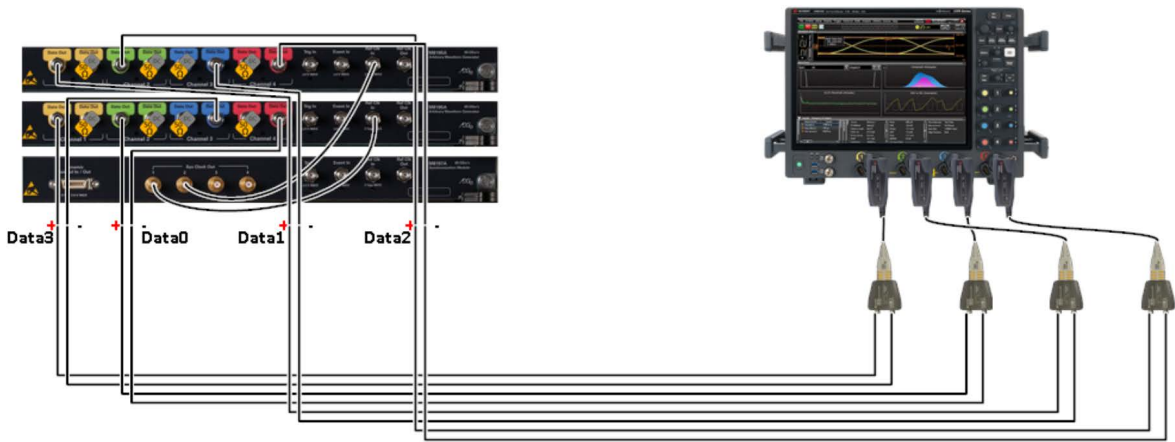
Figure 45 Example connection diagram for FRL Cable Random Jitter Calibration (terminated with scope probes)
