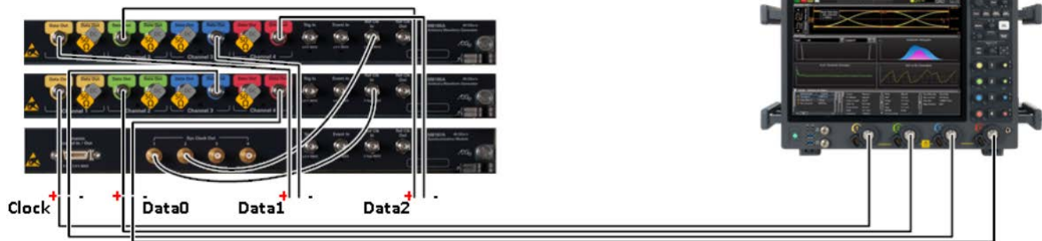
Figure 16 Example connection diagram for Sink Skew Calibration (connection 1)
