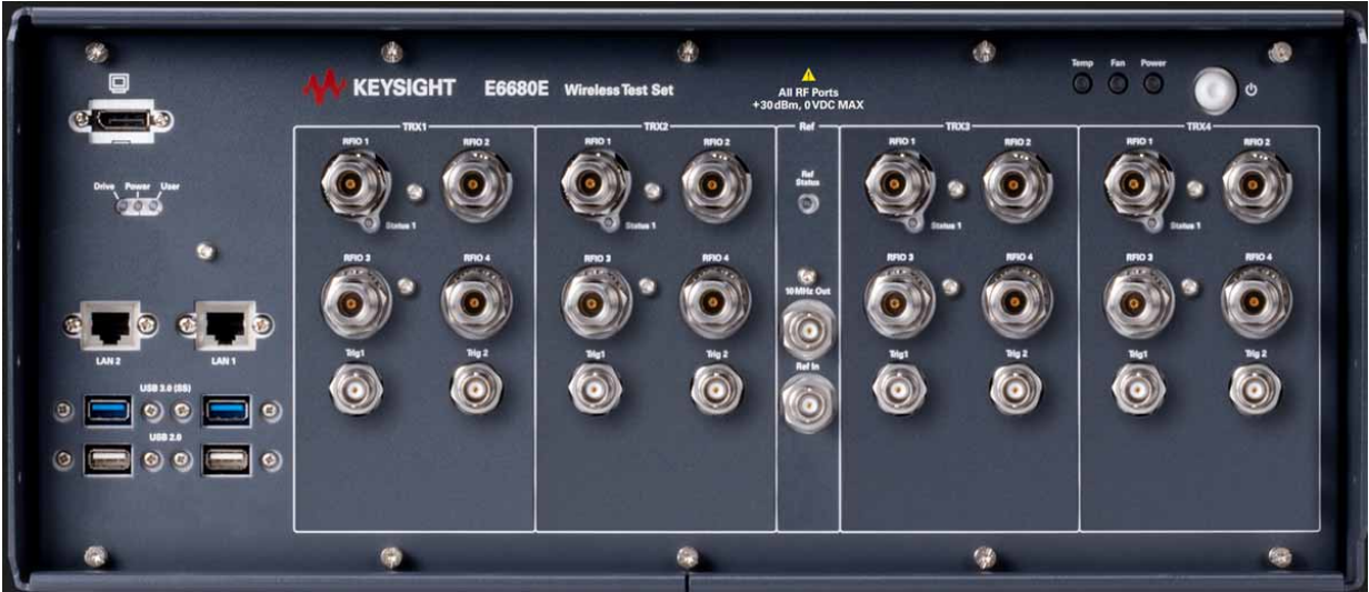
Figure 2-1 E6680E Front Panel
