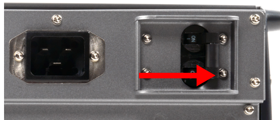
Figure 21 Chassis circuit breaker
