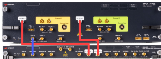
Figure 23 Two-channel system using one M8042A pattern generator (two channels) and one M8009A clock module
