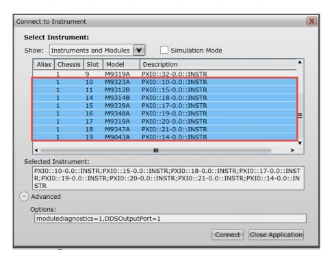
12.In the M9383B Soft Front Panel (SFP), select Utilities > Hardware Options Upgrade. Note that Single Channel VXGs may have modules spread out across the chassis slots.
