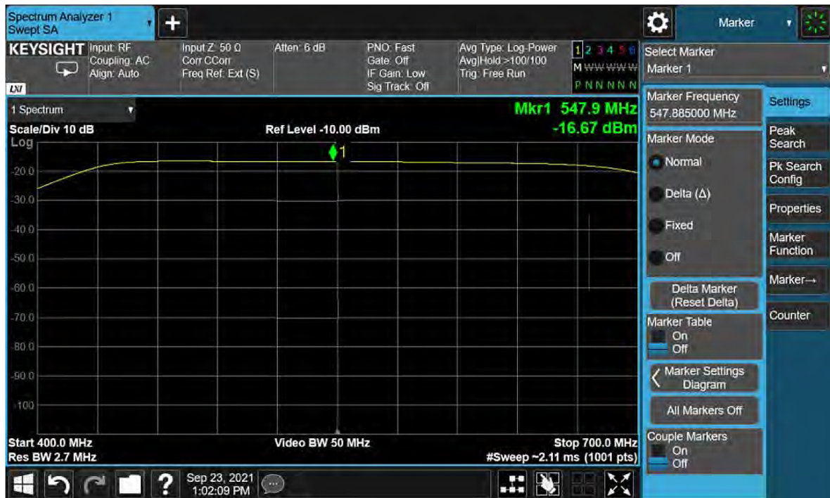
Figure 5-17 Band 8 Filter Shape
