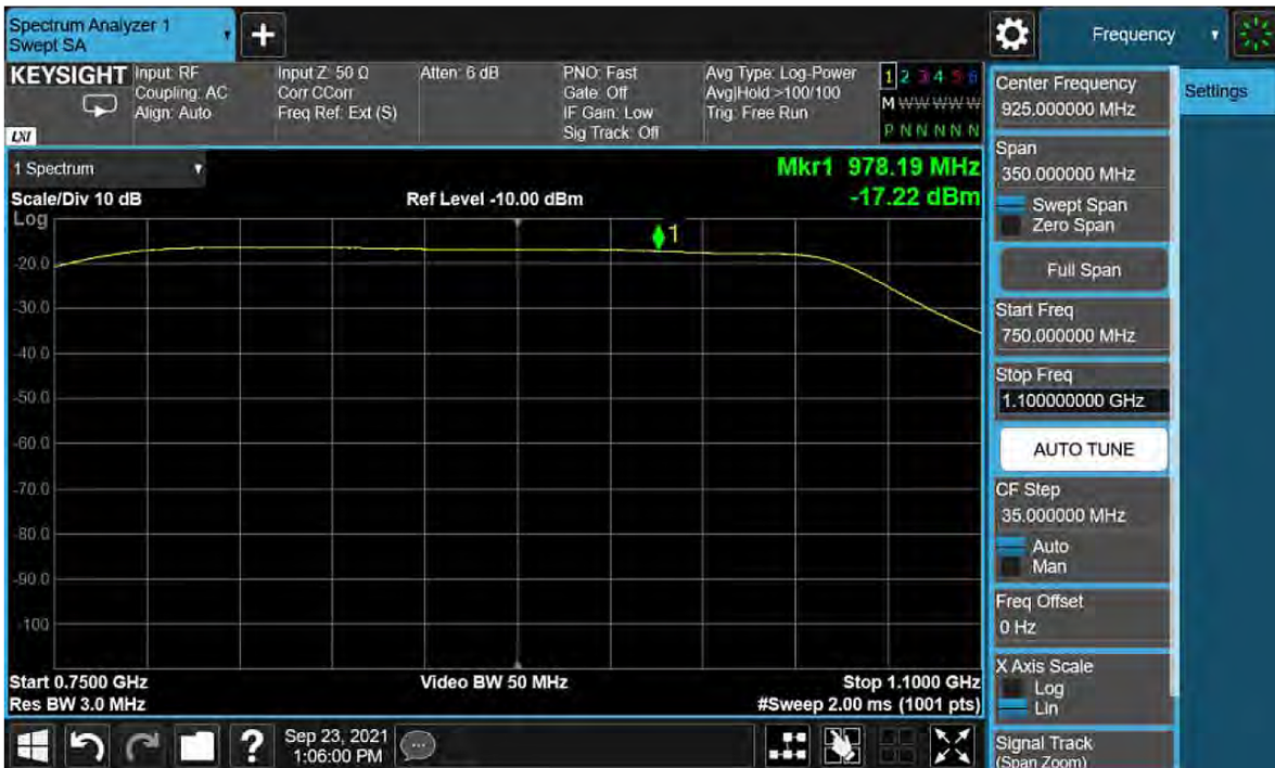
Figure 5-19 Band 10 Filter Shape
