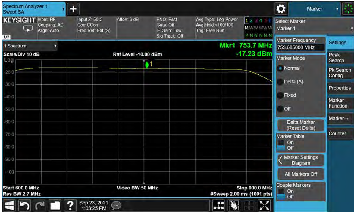
Figure 5-18 Band 9 Filter Shape
