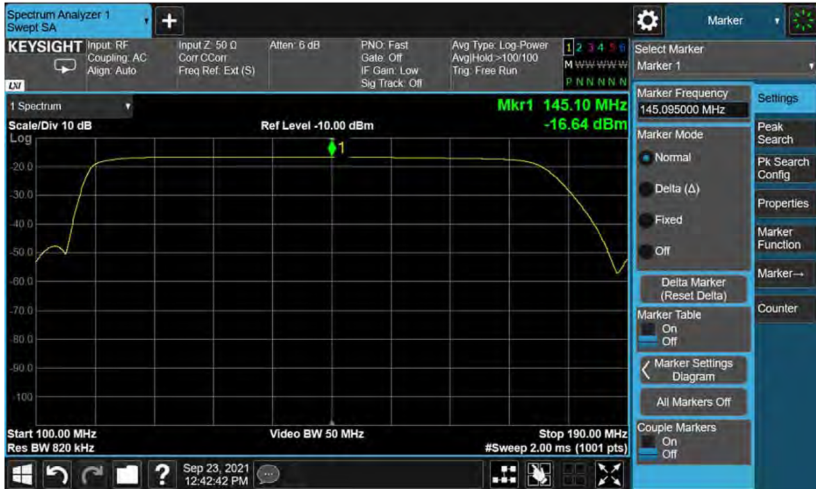
Figure 5-12 Band 3 Filter Shape
