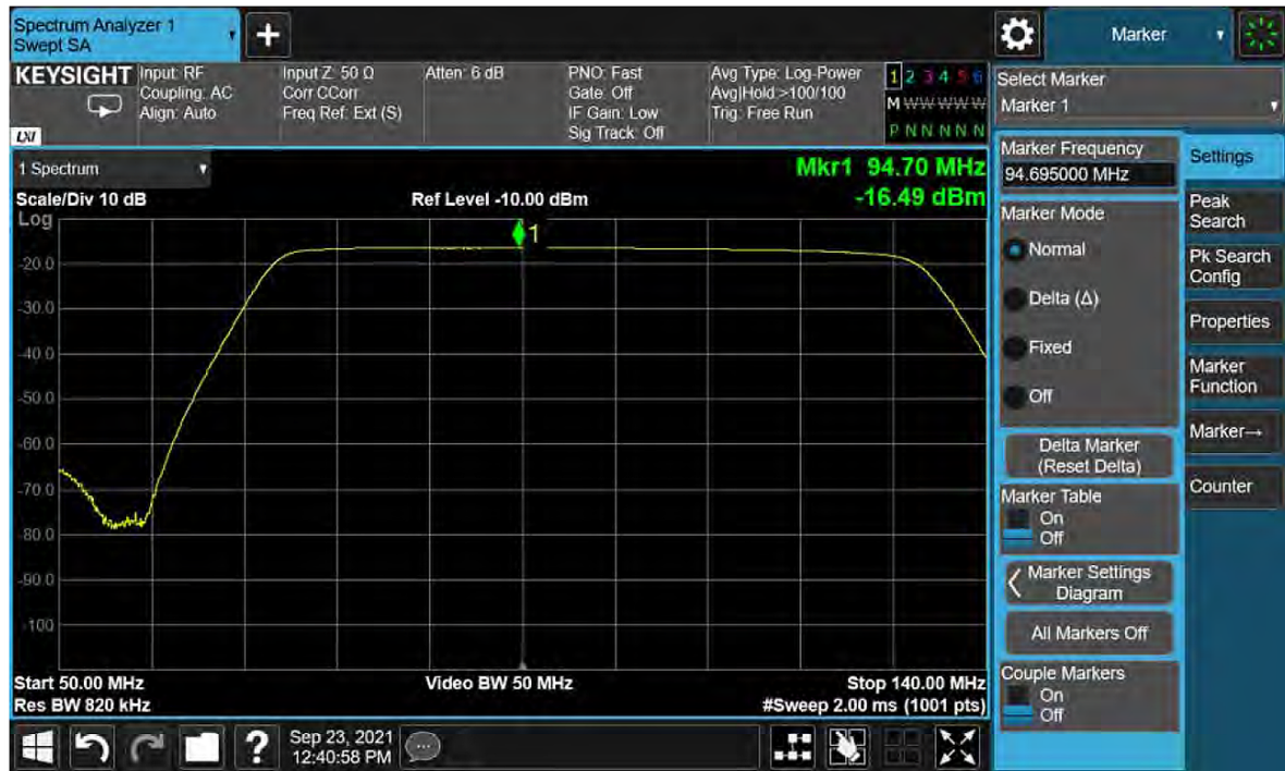
Figure 5-11 Band 2 Filter Shape
