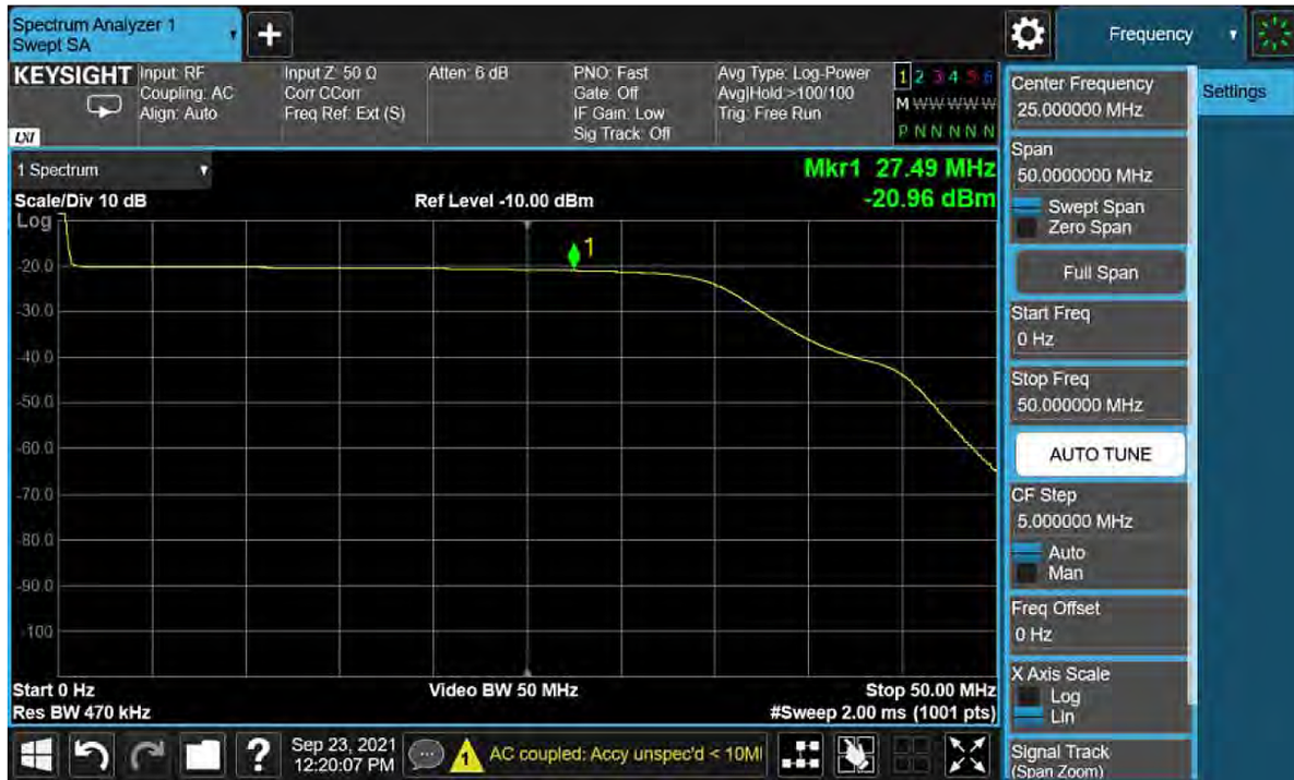
Figure 5-7 Band 1 Filter Shape
