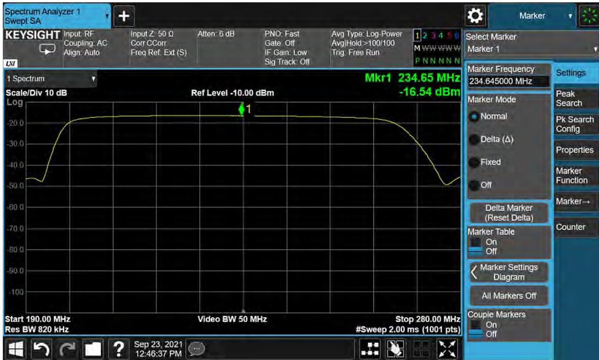
Figure 5-14 Band 5 Filter Shape
