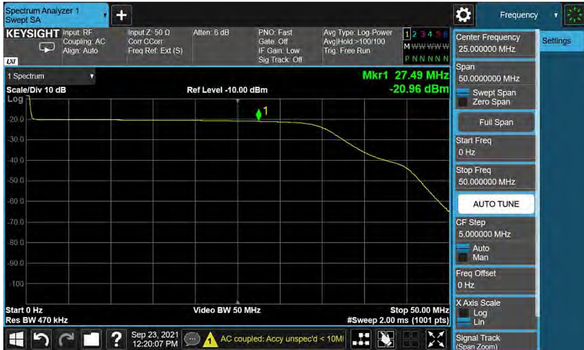
Figure 5-10 Band 1 Filter Shape
