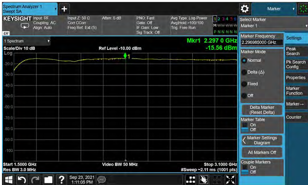
Figure 5-21 Band 12 Filter Shape
