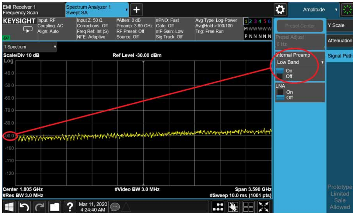
Figure 4-32 Internal Preamp Low Band Noise Floor Check
