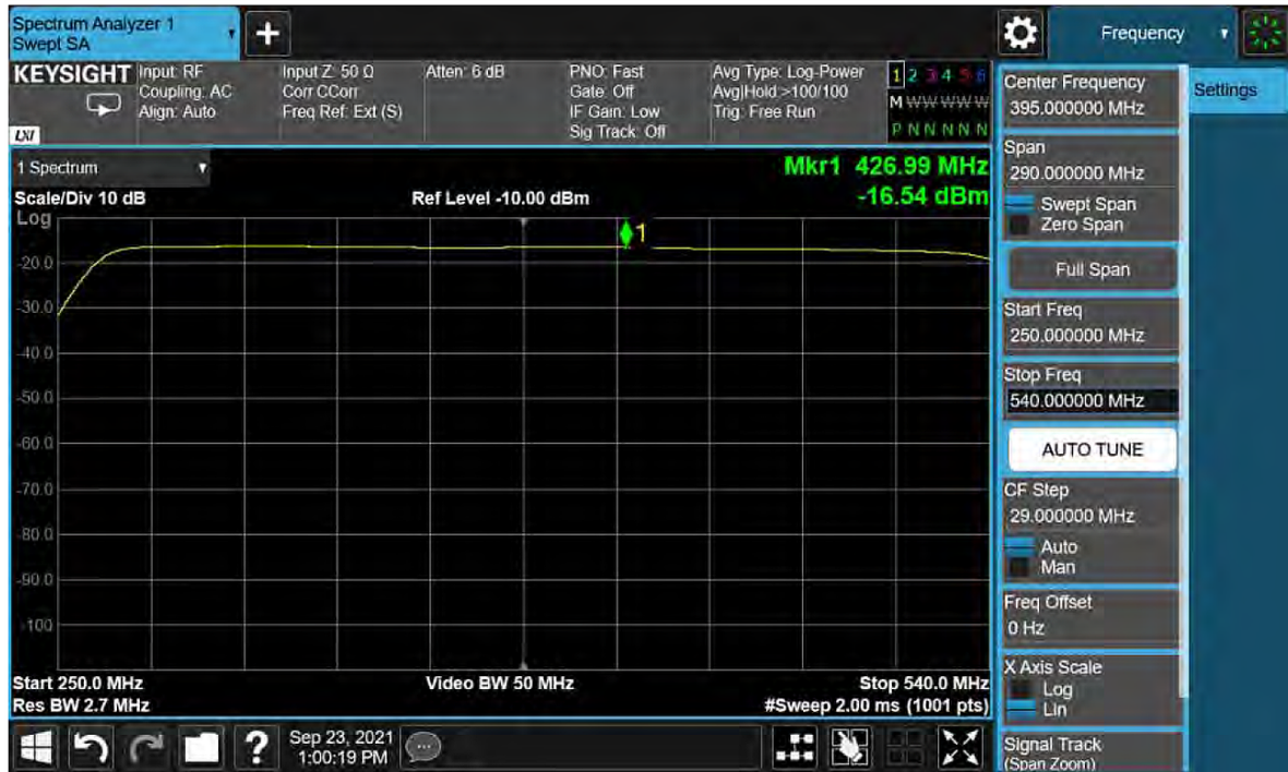
Figure 5-16 Band 7 Filter Shape
