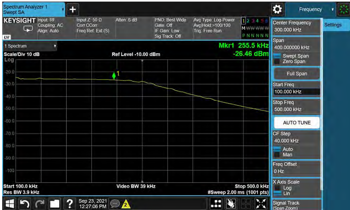
Figure 5-6 Band 0 Filter Shape
