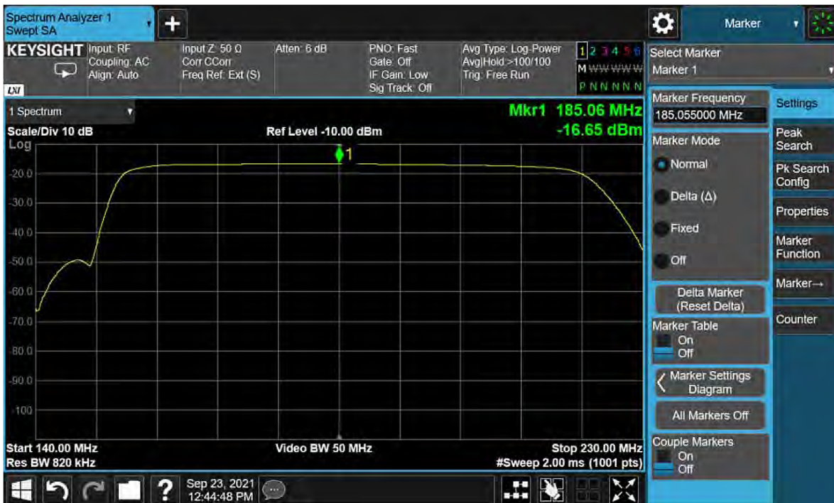
Figure 5-13 Band 4 Filter Shape
