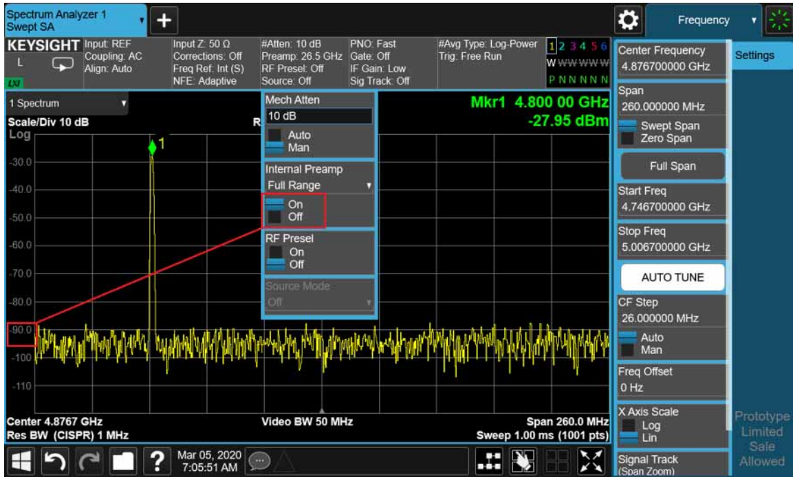
Figure 4-31 4.8 GHz Calibration Signal, Preamp On
