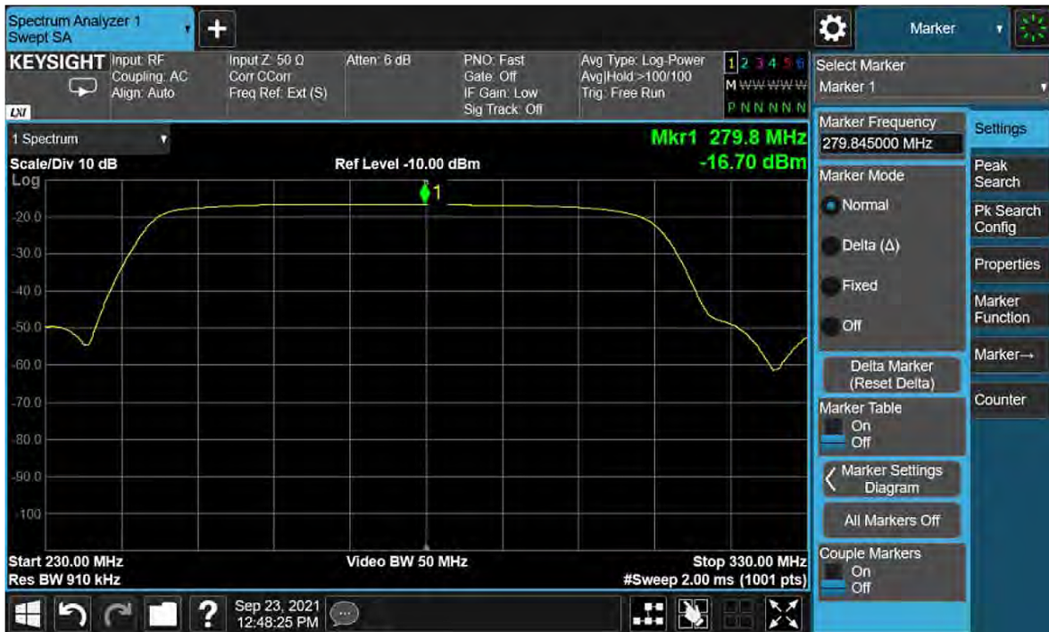
Figure 5-15 Band 6 Filter Shape
