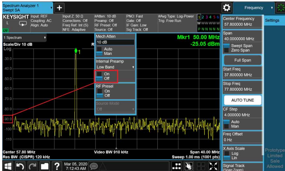
Figure 4-28 50 MHz Calibration Signal, Preamp Off
