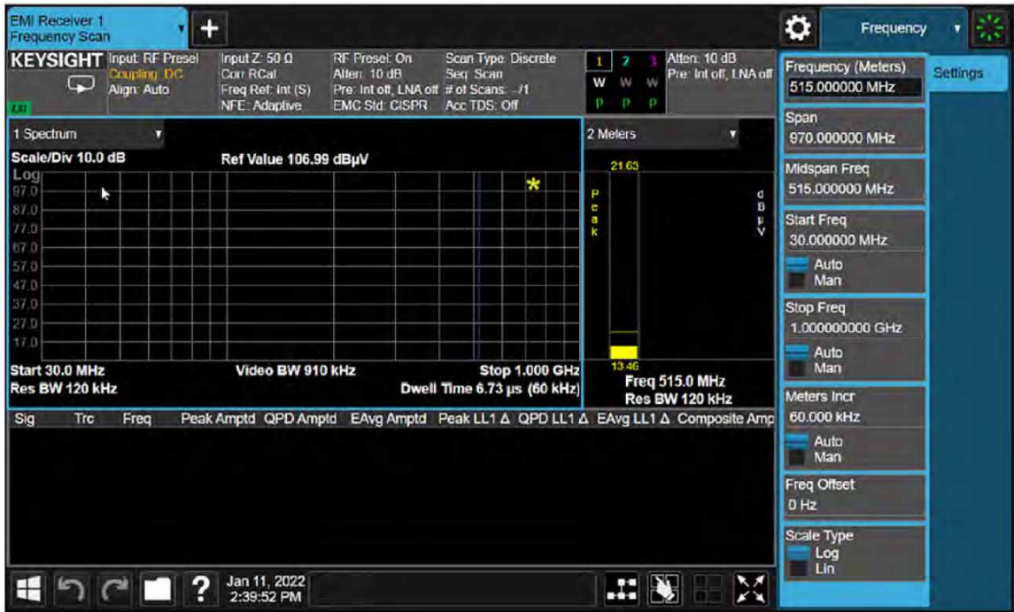
Figure 2-2 Typical Instrument State at Power-up
