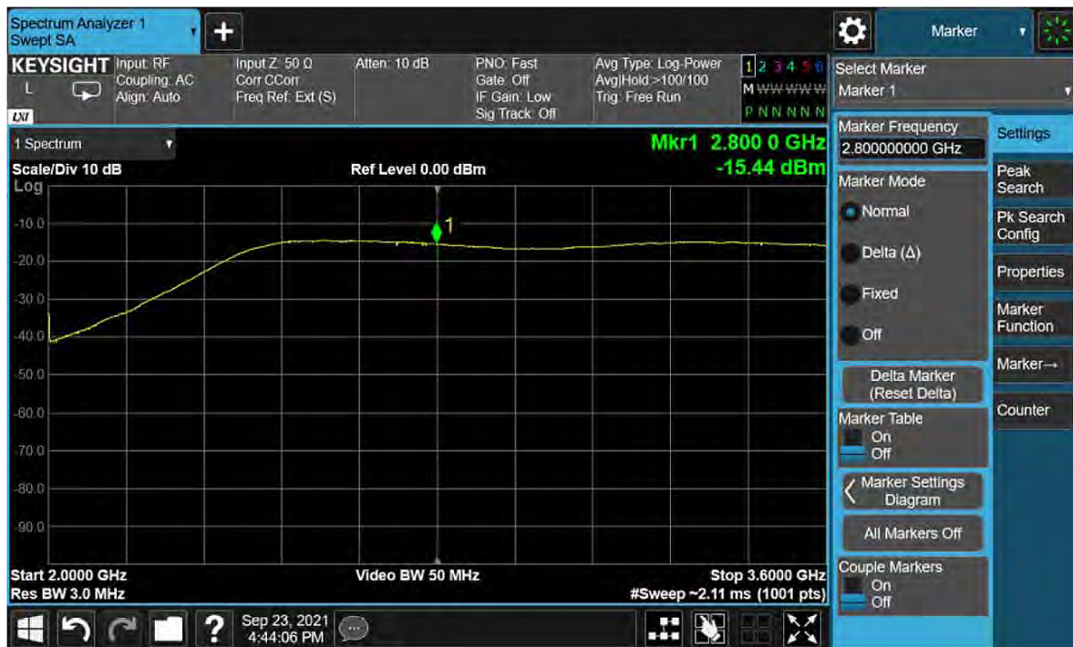
Figure 5-23 Band 13 Filter Shape
