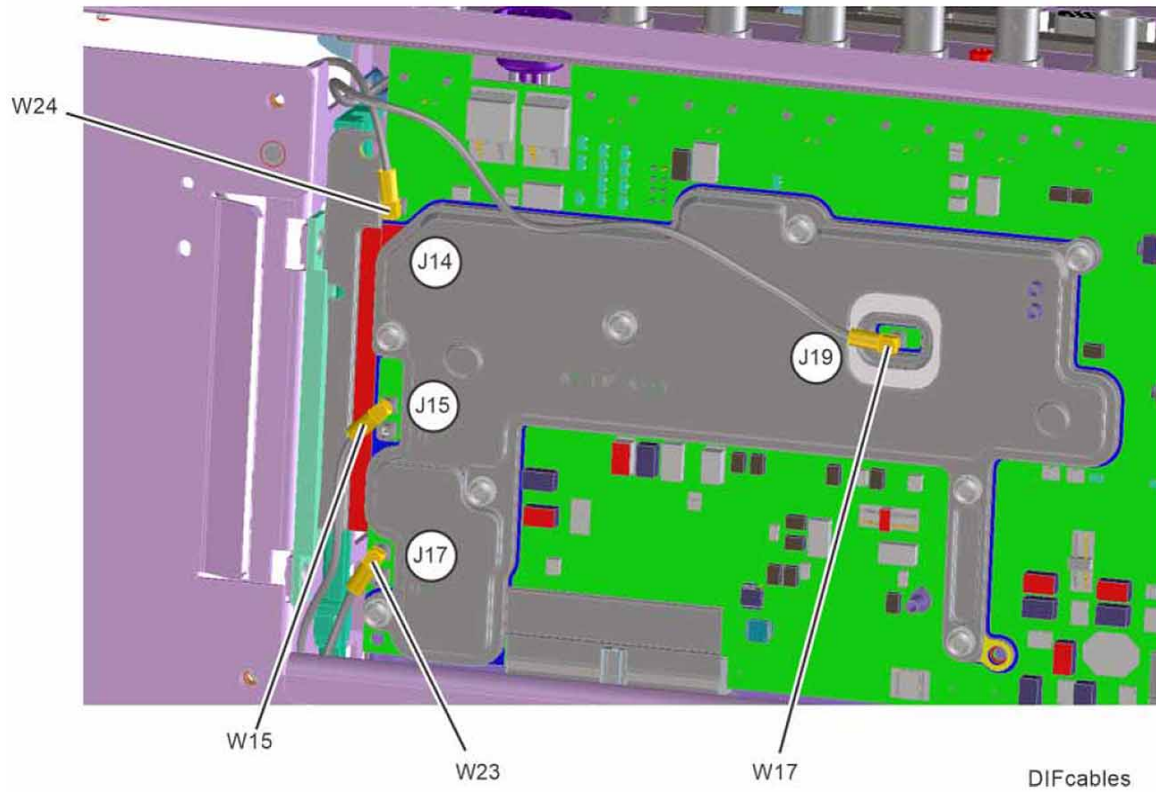
Figure 10-2 A3 Digital IF Assembly Cable Locations
