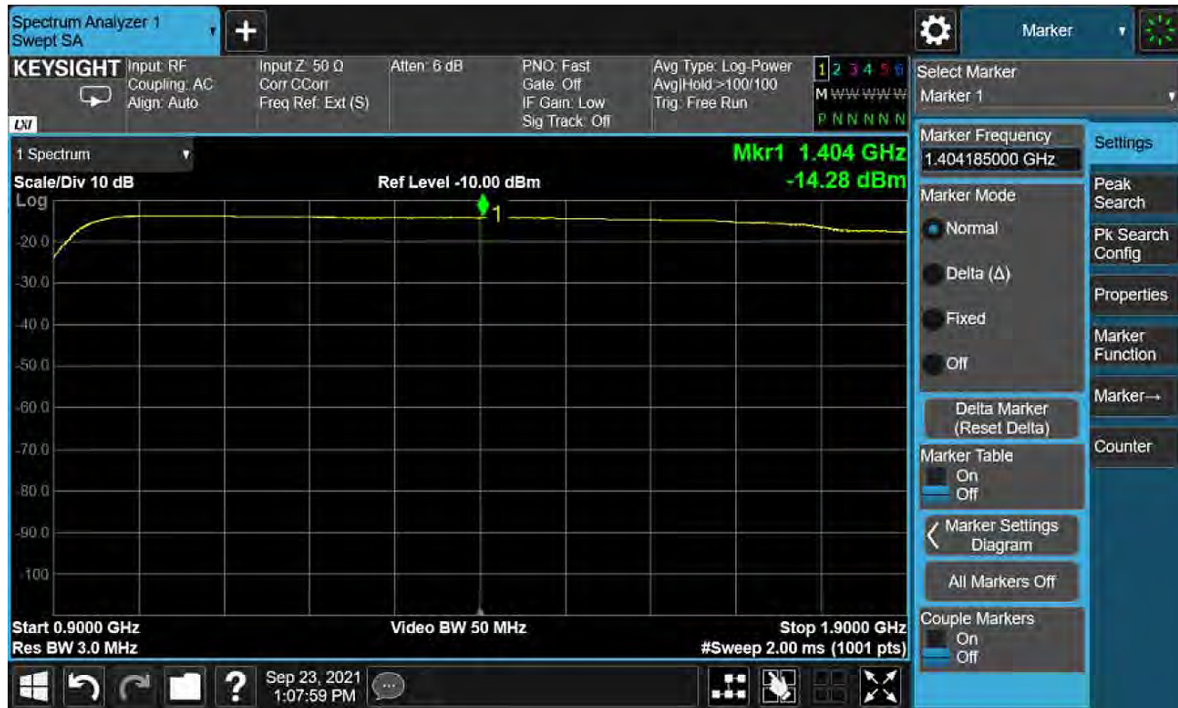
Figure 5-20 Band 11 Filter Shape
