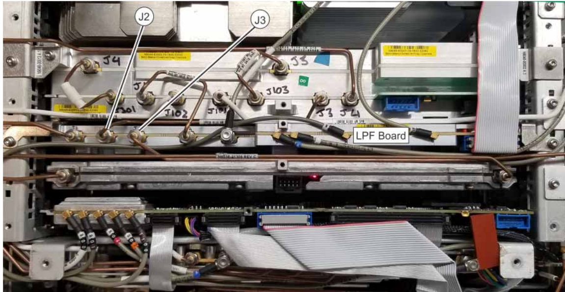
Figure 4-20 Cal Switch Connections Limiter Pre-Filter Board
