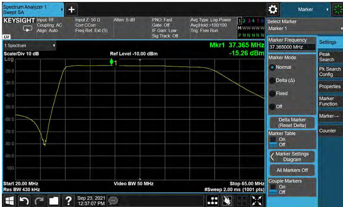
Figure 5-9 Band 0 Filter Shape
