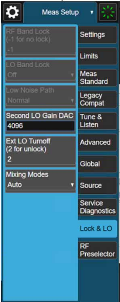
Figure 16-3 Lock and LO Menu (accessed via Spectrum Analyzer Mode --> Meas Setup --> Lock & LO)
