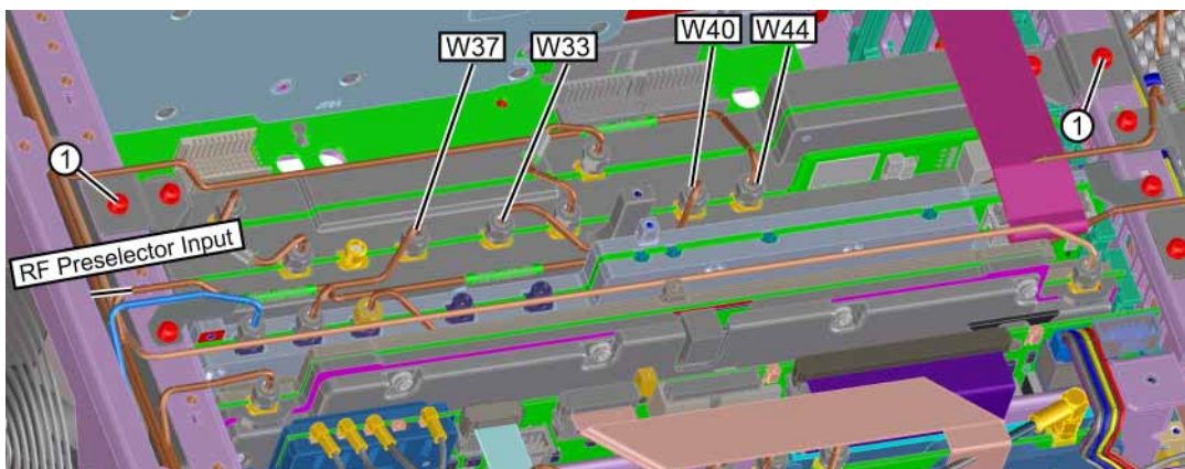
Figure 18-35 RF Preselector Cables
