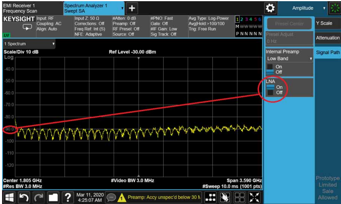
Figure 4-33 LNA Noise Floor Check
