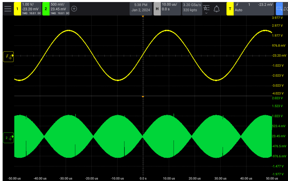
Figure 26 Amplitude Modulation Shown at 100% Intensity
