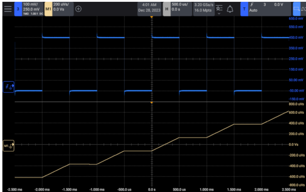
Figure 15 Integrate With Signal Offset
