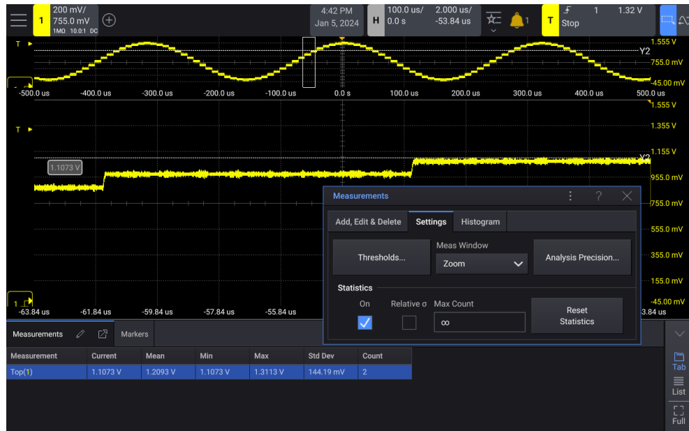
Figure 40 Isolating area for Top measurement
