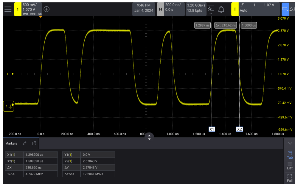
Figure 39 Moving the markers together to check pulse width variations
