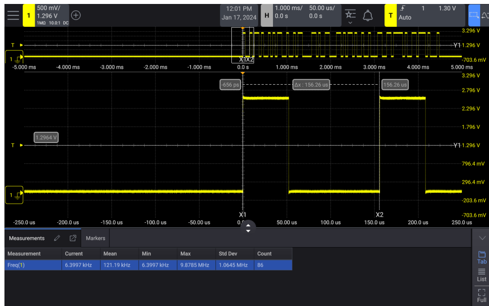
Figure 42 Isolating an event for Frequency measurement
