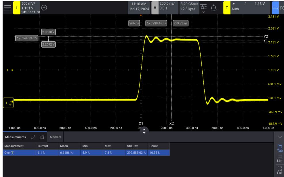
Figure 41 Automatic Overshoot measurement
