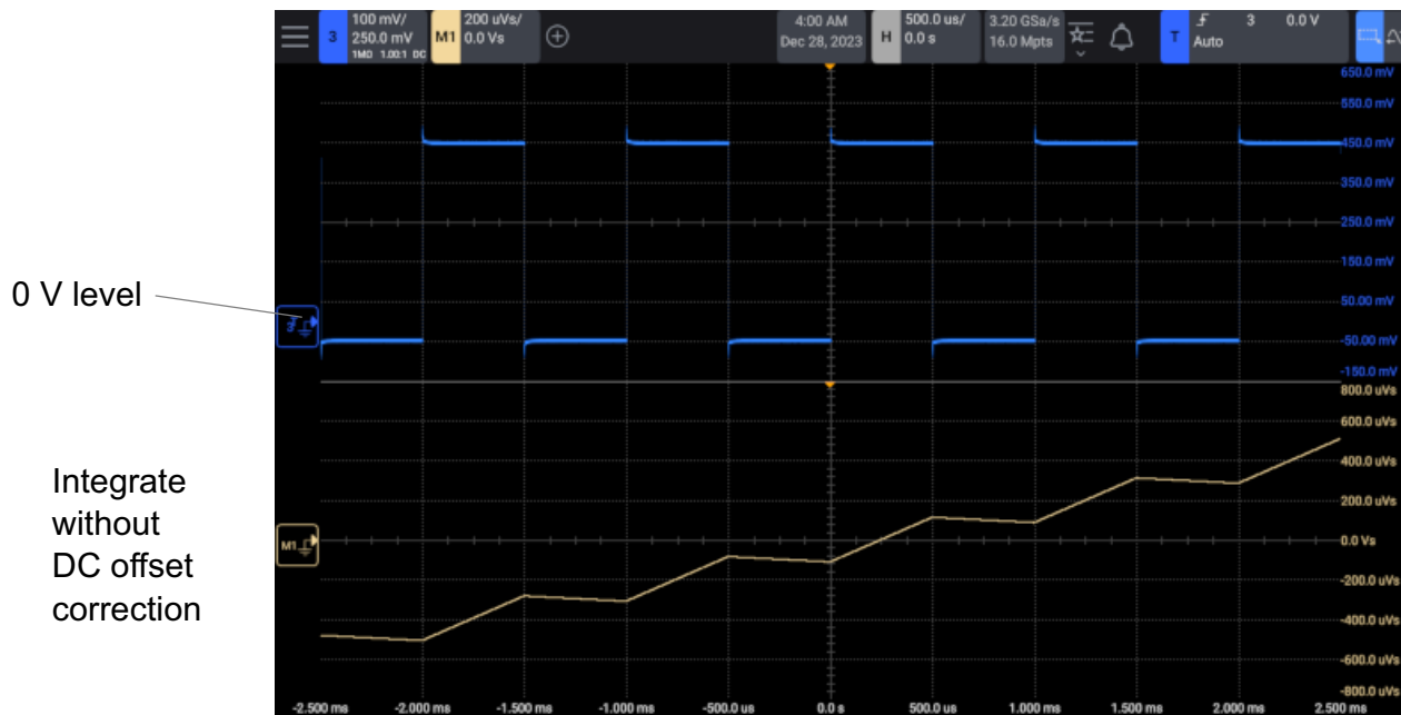
Figure 14 Integrate Without Signal Offset
