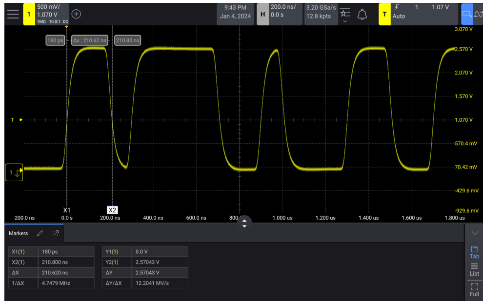
Figure 38 Measuring pulse width with markers
