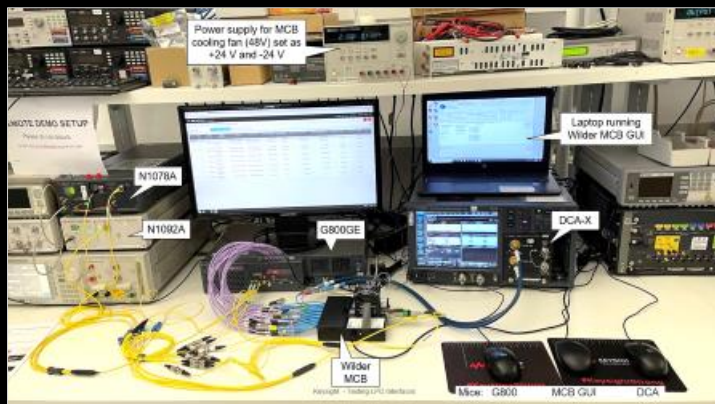
LPO setup in Keysight's lab
