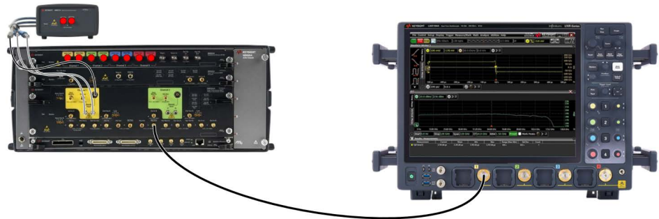
Figure 4-4 Example connection diagram for Reference Clock Calibration (M8040A)
