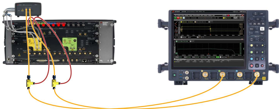
Figure 4-1 Example connection diagram for a terminated calibration procedure without an ISI trace (M8040A, 4-channel scope)
