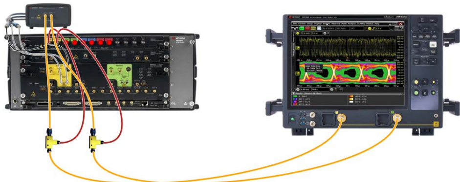
Figure 4-2 Example connection diagram for a terminated calibration procedure without an ISI trace (M8040A, 2-channel scope)
