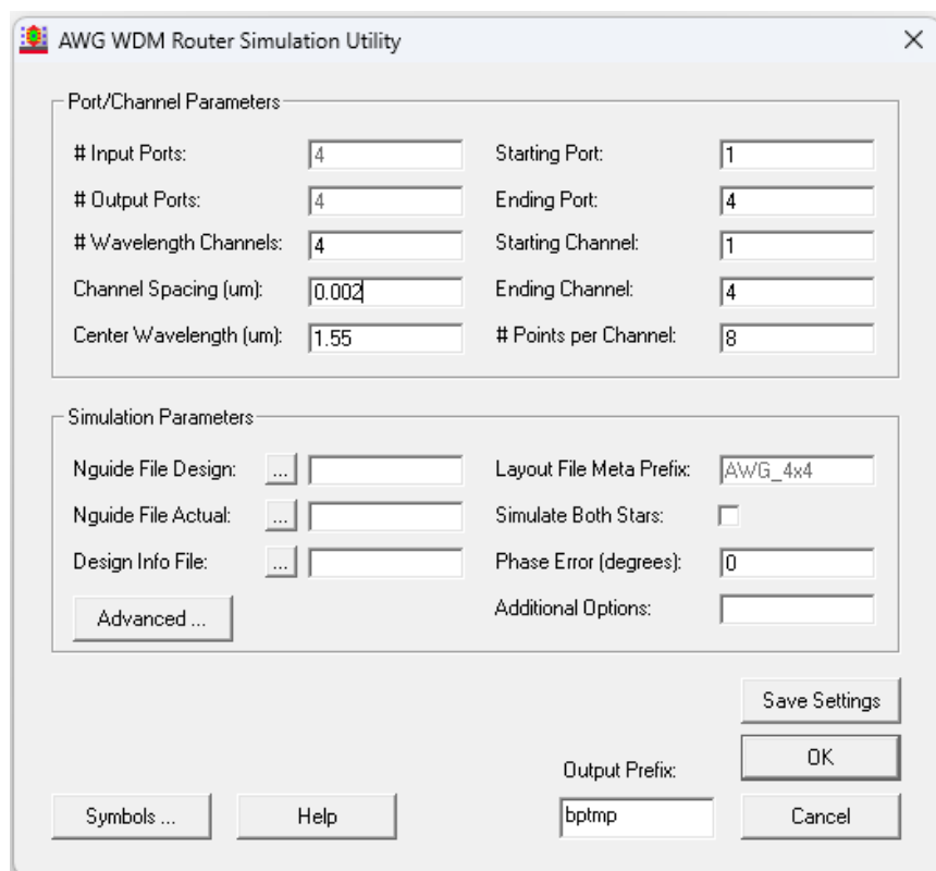
Figure 6. The AWG WDM Router Simulation Utility dialog, where two main sections are split including Port/Channel Parameters and Simulation Parameters.
