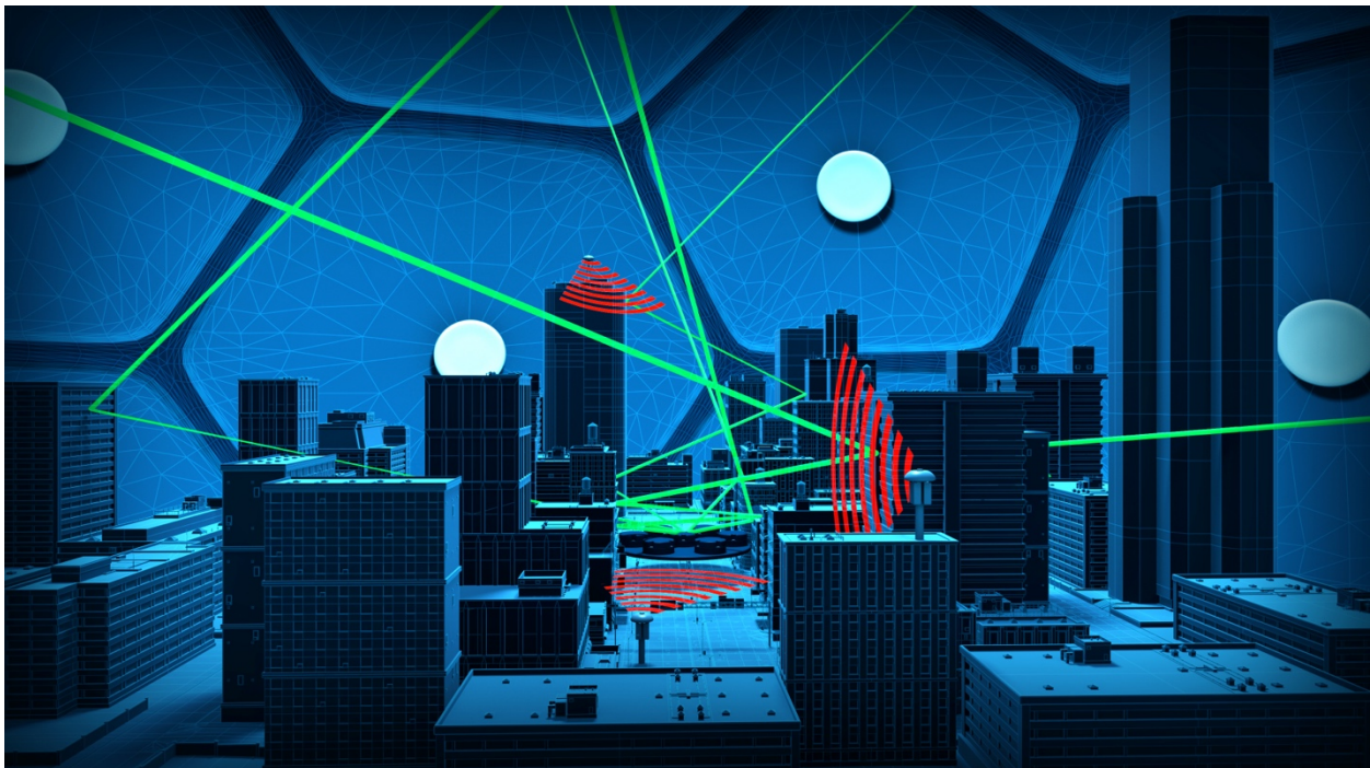
Illustration of a simulated test environment incorporating GNSS, multipath and jamming in a zoned chamber
