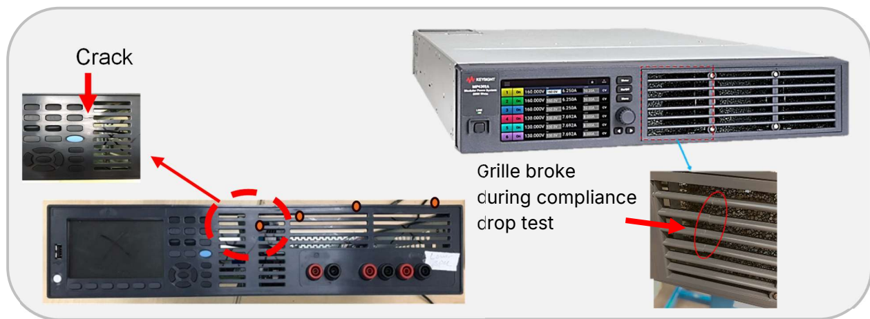
Figure 1. Instrument front housing damage during physical testing
