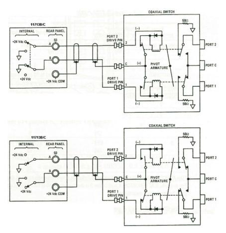
Figure 2-5 Typical connection for 8762 and 8765 series coaxial switches
