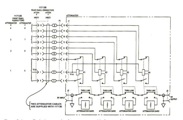
Figure 2-4 Typical connection for a programmable four-section attenuator
