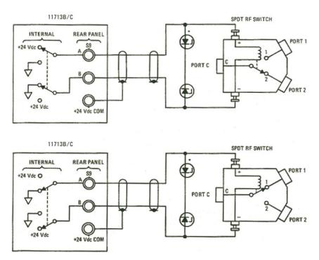
Figure 2-6 Typical connection for 8761 series coaxial switches
