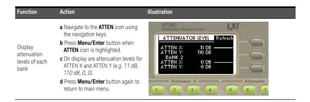
Attenuation value on display changes according to the input from the front panel pushbuttons or through the virtual web interface:
