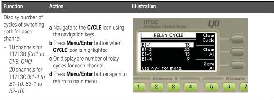
**a** Scroll to the desired bank-channel (e.g. B1-1) using the navigation keys.
