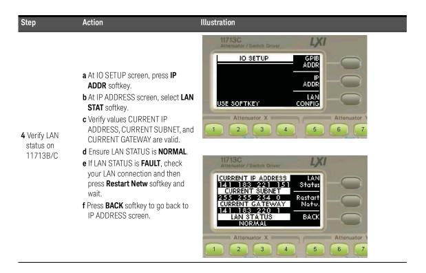
Now you can use the 11713B/C Web Browser Interface to access and control the instrument. See "Exploring the 11713B/C Web Interface over LAN" on page 79.
