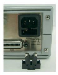
**3** Remove fuse and replace with one of the correct rating and type for your selected input ac line voltage.
