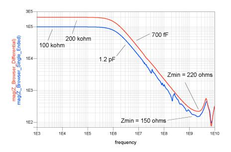
Figure 29 Input Impedance (Differential)
