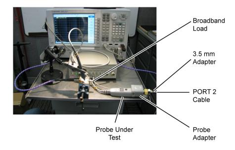
Figure 49 Measurement Setup for Vout
