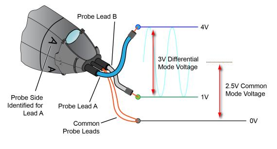
Figure 9 Example InfiniiMode Probe Circuit Connections
