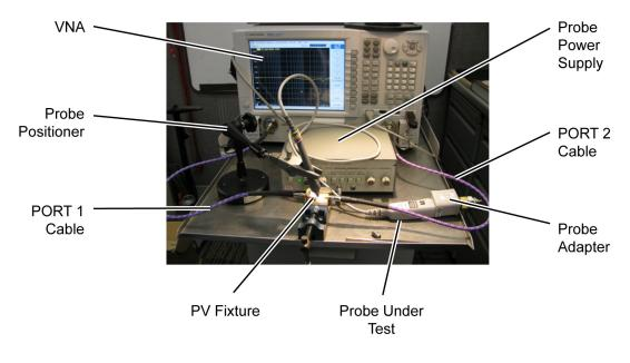
Figure 46 Measurement setup for V<sub>in</sub>
