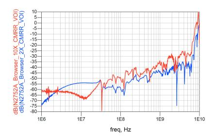
Figure 25 CMRR, Differential (2:1 and 10:1 Attenuation)
