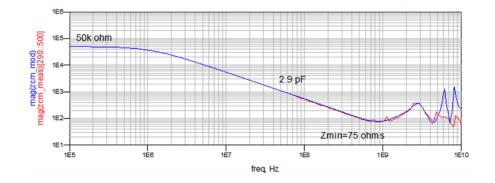
Figure 19 Common Mode Input Impedance (Measured, Modeled)
