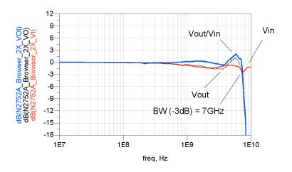
Figure 24 Frequency Response (Differential)
