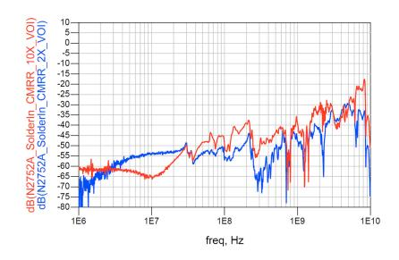
Figure 34 CMRR, Differential (2:1 and 10:1 Attenuation)
