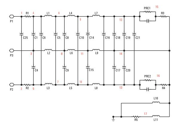
This model should be viewed as a black box model. While it is somewhat physically based, the response has been optimized so it accurately reflects the port impedances so component values may not agree totally with the actual physical implementation.
