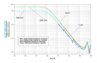
The SPICE model for the green "Modeled" plot shown in **Figure 30** below is described in **"N2752A probe with the N2776A Browser Tip**" on page 30.
