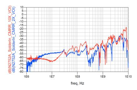
Figure 37 CMRR, Differential (10:1 and 2:1 Attenuation)
