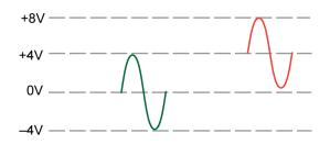
Figure 8 Vertical Offset Applied to an Input Signal
