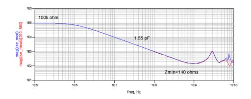
Figure 17 Single-Ended Input Impedance (Measured, Modeled)
