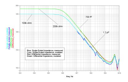
Figure 14 Input Impedance, Measured and Modeled (Differential)
