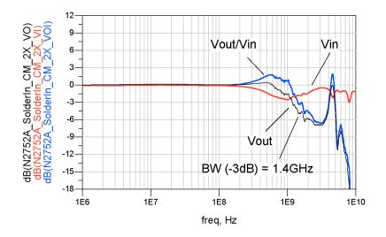
Figure 35 Frequency Response (Common Mode)
