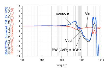
Figure 40 Frequency Response (Common Mode)
