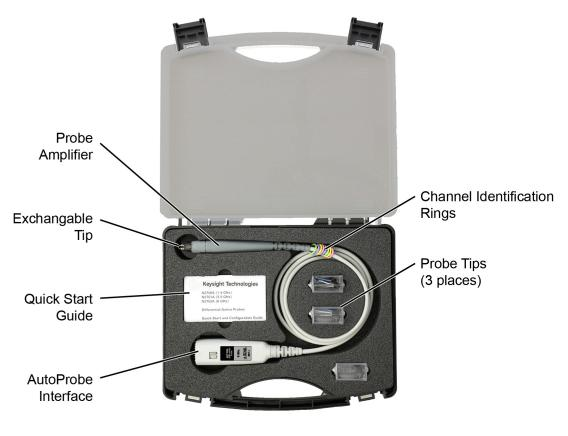
Figure 1 Probe with Supplied Accessories and Case
