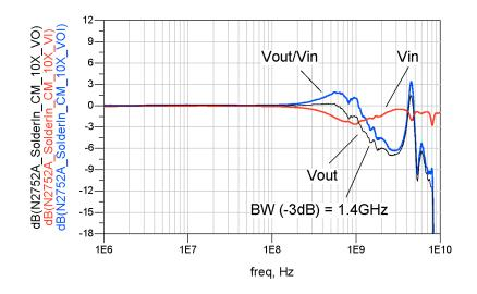
Figure 38 Frequency Response (Common Mode)
