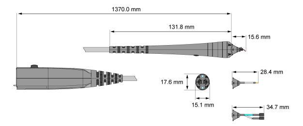
Figure 22 Probe and Tip Dimensions
