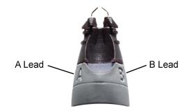
Figure 10 Lead Identification on Probe Body
