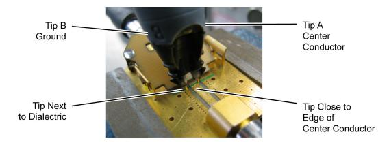
Figure 47 Close-Up Showing Tip Spacing and Position
