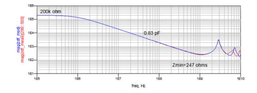
Figure 18 Differential Input Impedance (Measured, Modeled)
