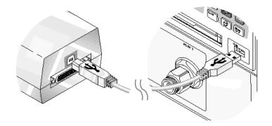
Figure 43 Connecting Calibration Module's USB Cable
