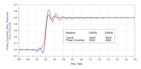
Figure 26 Time Response to an Ideal Steip at Probe Tip (Differential) (Step Response)
