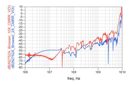
Figure 32 CMRR, Differential (10:1 and 2:1 Attenuation)
