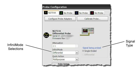
Figure 11 Probe Configuration Dialog Box
