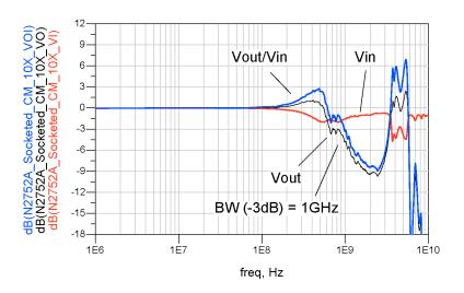
Figure 42 Frequency Response (Common Mode)
