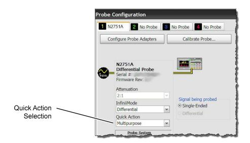
Figure 12 Probe Configuration Dialog Box
