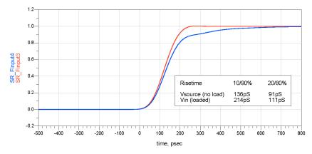
Red. V<sub>source</sub>: Differential 100 ohm source (source and load terminated) with no load applied. Blue. V<sub>in</sub>: Same source with N2752A loading applied.
