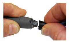
Figure 4 Aligning the Tip to the Probe
