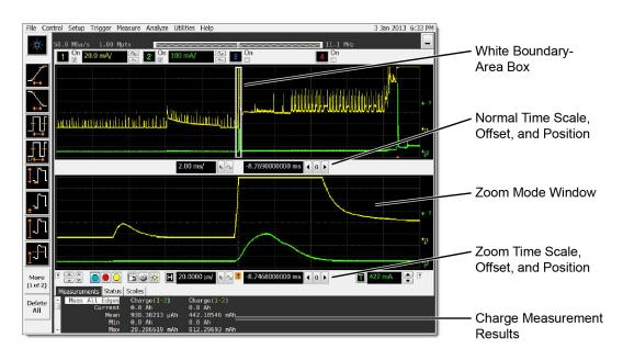
Figure 12 Charge Measurement of Mobile Phone Current in Standby State with Zoom Mode
