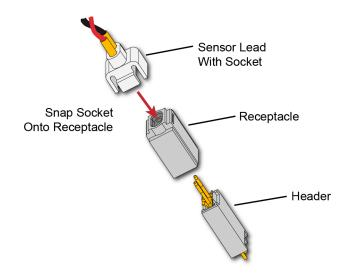
Figure 17 Socketed Lead Snaps Onto the MBB Receptacle
