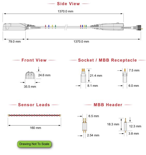
Figure 42 Probe and Tip Dimensions
