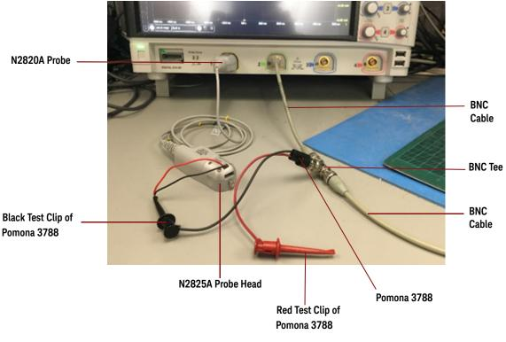
Figure 30 Example of Initial Calibration Setup
