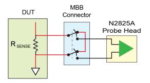
Figure 19 MBB Connector With N2825A User-Defined Head
