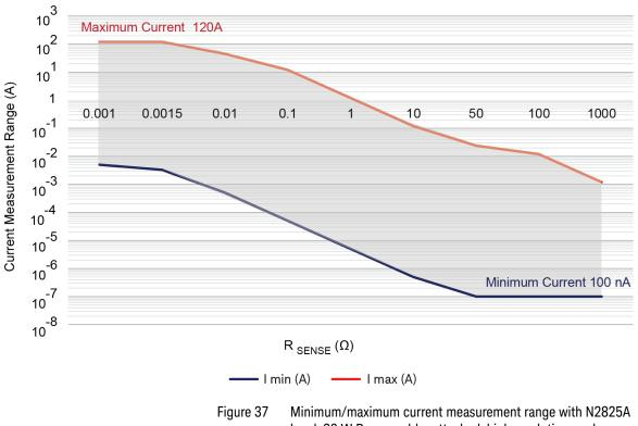
head, 20 W  $\mathrm{R}_{\mathrm{sense}}$ , solder attached, high resolution mode on
