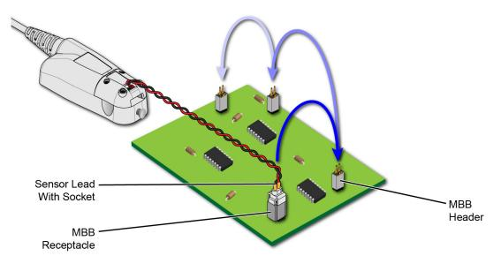
Figure 16 Probing with MBB Connector on DUT
