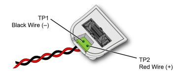
Figure 5 Lead Positions on PC Board
