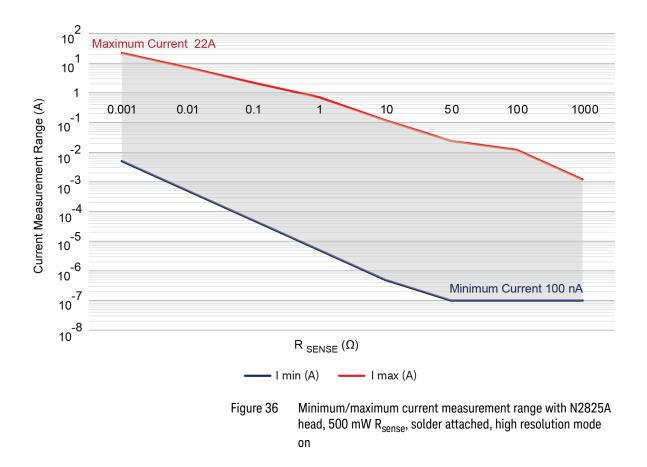
5 Characteristics and Specifications Current Range Vs. R<sub>SENSE</sub> Graphs
