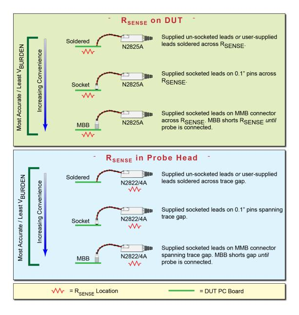
Figure 3 Different Probing Connections With Relative Merit
