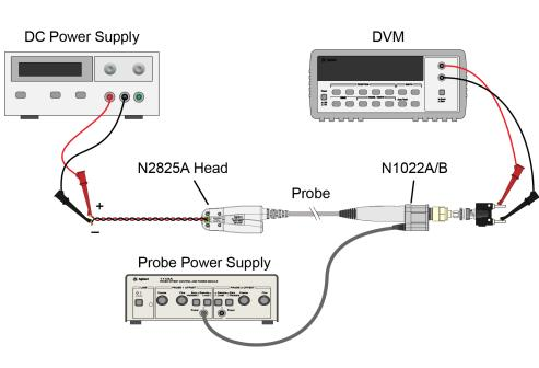
Figure 52 Test Setup for Measuring Vout
