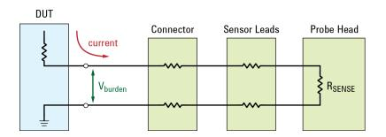
Figure 20 V<sub>burden</sub> Developed Across Probing Components
