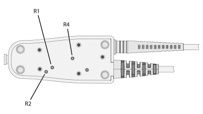
Figure 32 Location of Calibration Adjustments
