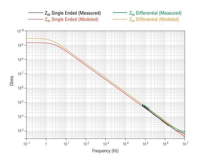
Figure 49 Input Impedance
