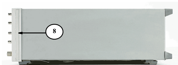
Figure 2-36 Trim-Side Overlay (Installed)
